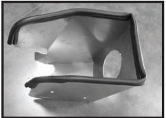
Step 9 Install bulb seal around edges of heat shield as shown.
