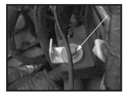
Step 8 Install battery side bracket using hardware that was emoved in step 6.
