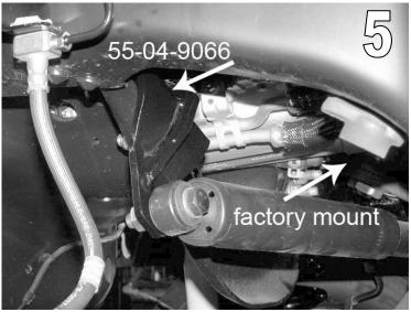
fasten with the supplied 1/2" hardware. Attach the stabilizer to the steering stabilizer bracket (#55-04-9066) and tighten until bushings swell slightly.
