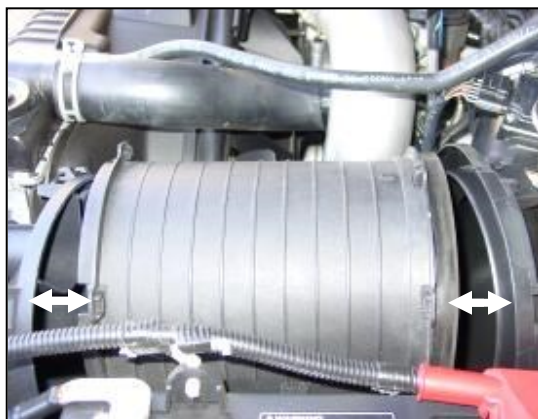
2. Remove the factory airbox by separating the inlet and outlet sections of the assembly.
