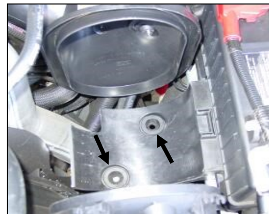
3. The factory airbox is held in place by two rubber grommets. Pull straight up and remove the box. (Note: make sure the factory grommets remain in the lower airbox support.)
