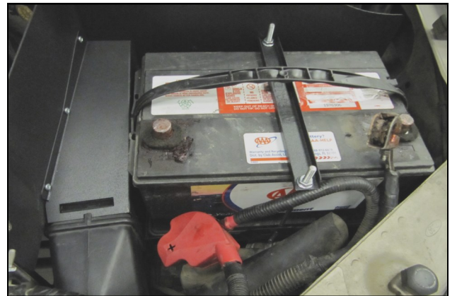
15. Secure the battery in place using the new 1/4-20 J Bolts (#11), Tie Down (#8) and 1/4-20 Flange nuts. The CAD Panels are slotted to accommodate the J Bolts.
