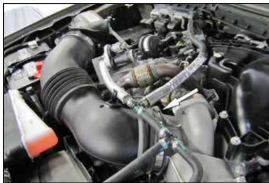
3. Loosen the hose clamp that secures the factory intake tube to the turbo inlet, release the four clips that secure the upper air filter housing and then remove the assembly from the vehicle.
