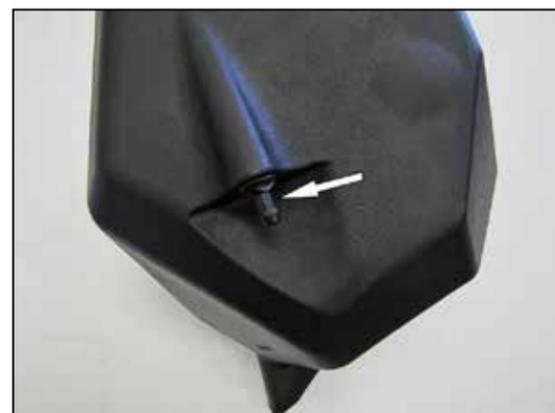
6. Install the provided air box mounting stud onto the AIRAID® housing using the provided hardware.
