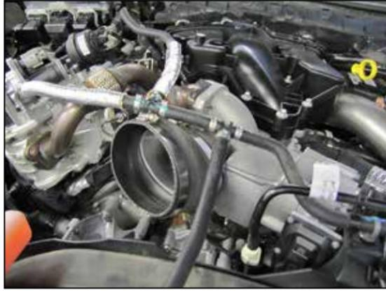
10. Install the provided coupler (08695) onto the turbo inlet and secure with the provided hose clamp.
