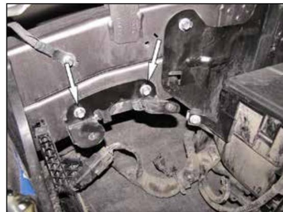
5. Remove the two bolts that secure the air filter housing mounting bracket to the inner fender and remove the bracket from the vehicle.
