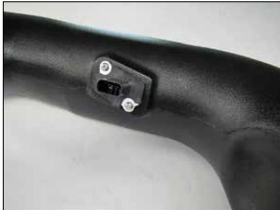
11. Remove the mass air sensor from the factory air filter housing and install it into the AIRAID® intake tube using the provided hardware and spacers. Install the AIRAID® decal onto the intake tube.
