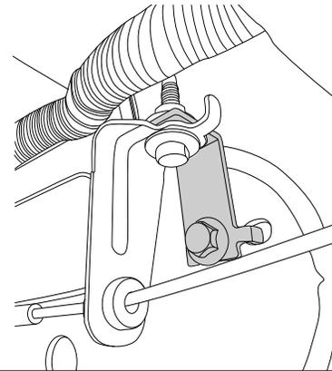
Locate mounting points; first and last set of studs on the inner sill. Motor Linkage mounts toward the front of the truck and Idler mount toward the rear. Driver side shown below.
