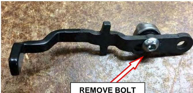
8. Remove bearing and bolt from latch assembly.
