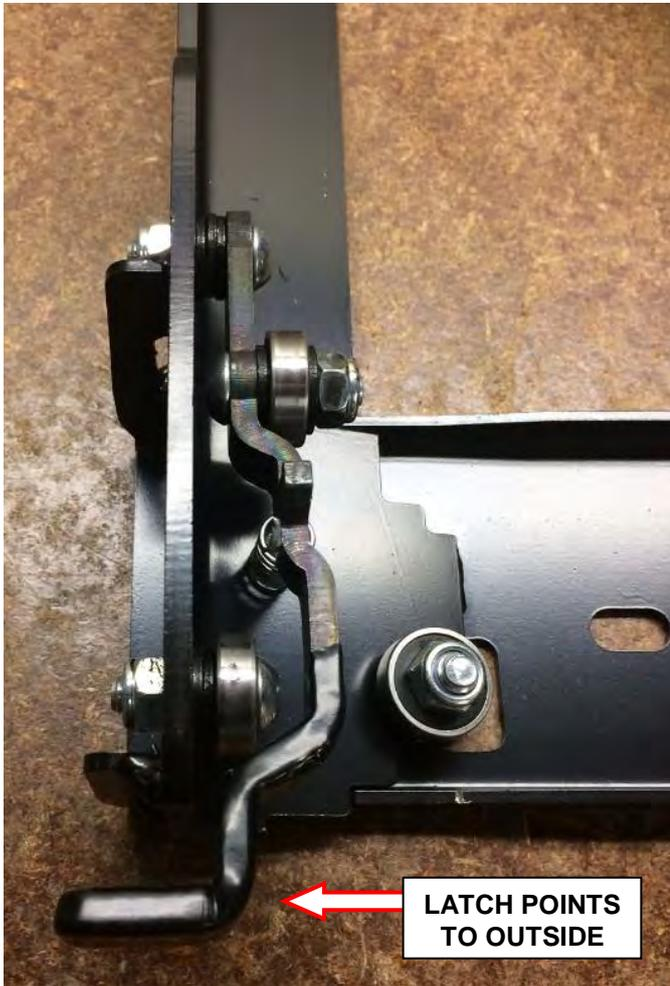
10. Rotate the latch and install it into the corresponding hole on the opposite side of the fridge slide frame. The plastic dipped handle should now be pointing towards the outside of the fridge slide as shown.
