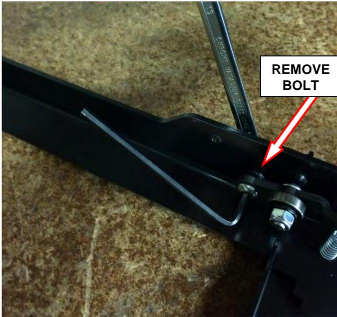
7. Remove the latch by removing the M8 x 25mm bolt, nut and washers using a 13mm ring spanner and 5.0mm hex key as shown.
