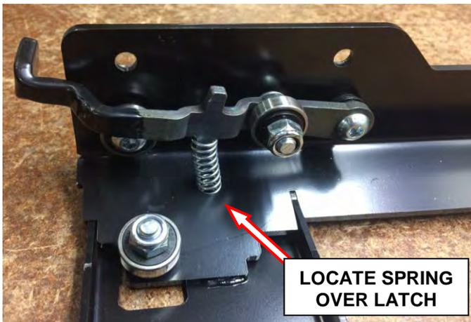
13. With the latch in the vertical position, install the spring into the hole as shown.
