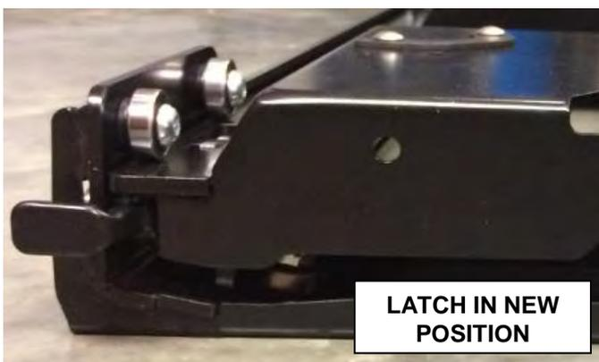
17. Refit the 4 rollers removed in Step 2. Tighten bolts to the recommended torque.
