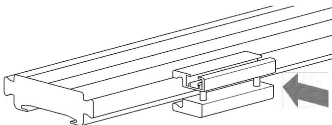
2. Loosen the M6 screws and slide over the BASE RACK dovetail
