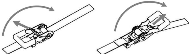
16. To release the bottle, release tension on the ratchet strap
