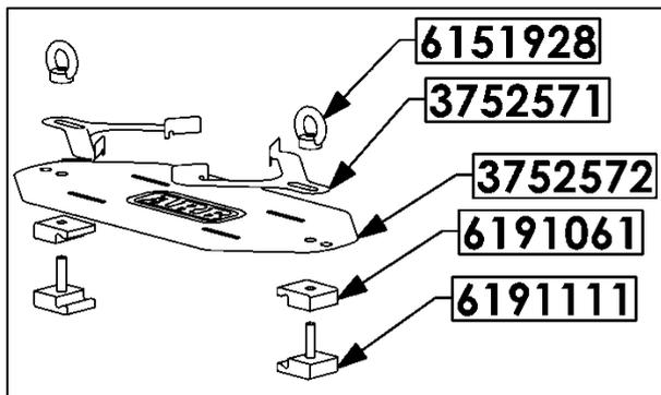
4. Fit the clamps and eye nuts as shown, into the inner or outer holes (to suit bottle size above)
