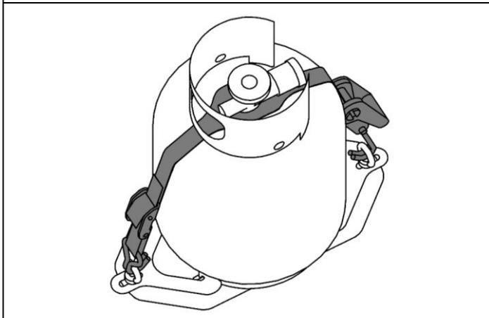
12. Engage the cam buckle and ratchet end hooks into the eye nuts
