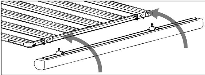
8. Fit the awning by placing the flange nuts and studs through the large hole, slide forward or backward to fully engage
