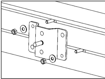
7. Use the awning fasteners to fix the awning brackets to the awning, at the same spacing as step 3.
