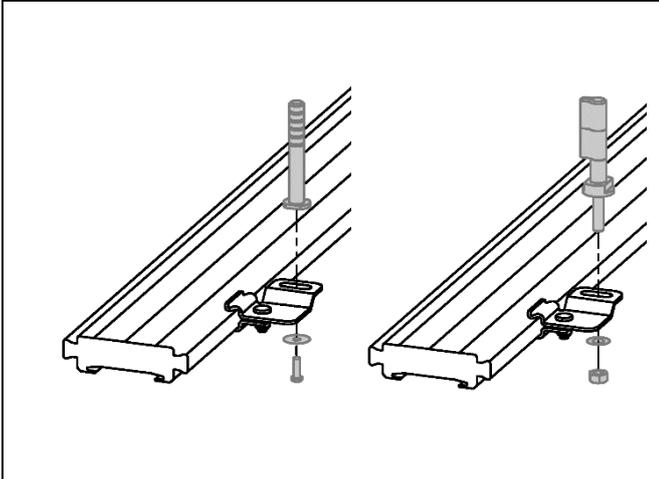
3. Loosely install the mounting pins as per manufacturer's instructions
