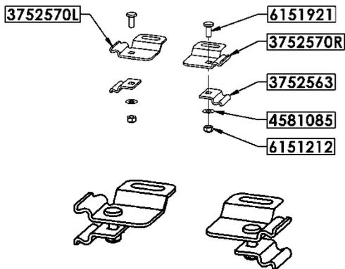
1. Assemble brackets with a pair of M8 bolts, washers and nuts
