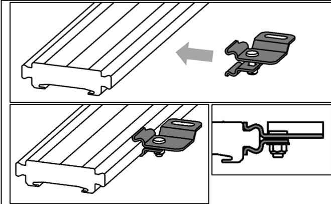
2. Fit the mounting brackets over the dovetail. Loosely tighten
