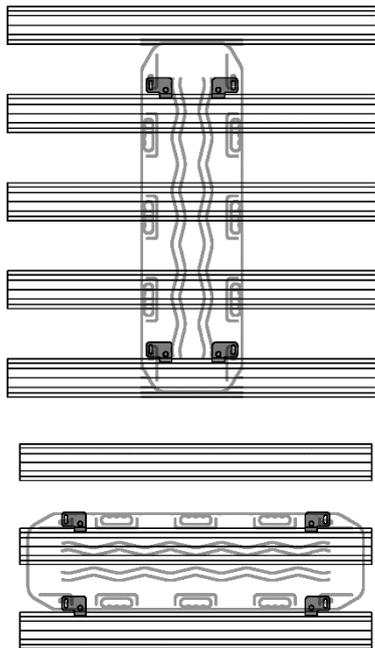
3. MAXTRAX bracket location for longitudinal and lateral mounting
