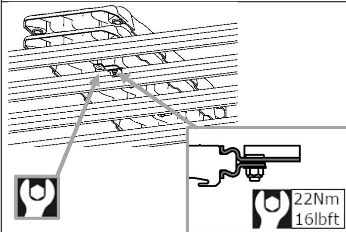
5. Tighten the M8 nut as per specified torque
