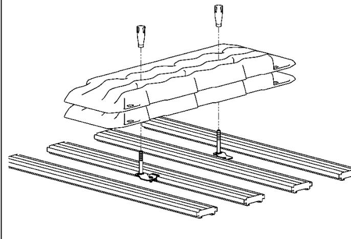
4. Fit the recovery boards to the pins to confirm locations
