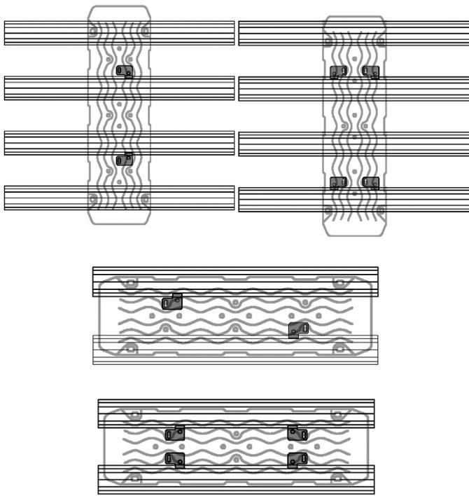
2. TRED Pro™ bracket location for longitudinal and lateral mounting, with 2 or 4 brackets is shown
