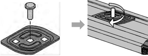
6. Using ARB Part No 6980060 (supplied separately), install the M8 stud into the stud plate as shown
