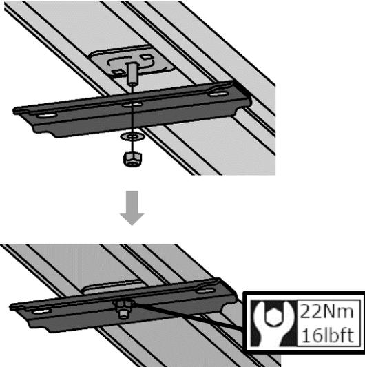
8. Install the bridging plate on to the stud, using an M8 nut and washer
