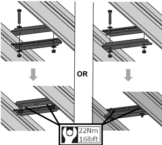
4. Place the clamps between two BASE Rack Cross beams, with one on either side of the dovetail
