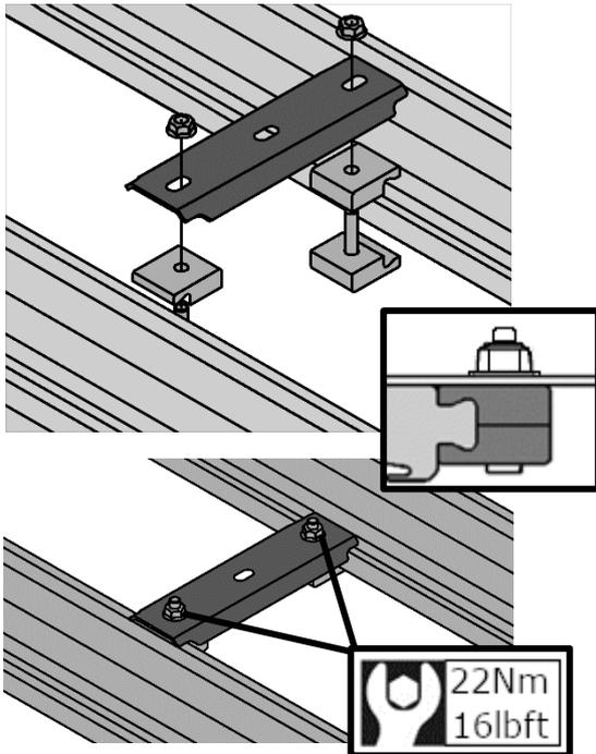
10. Arrange the alloy mount blocks (ARB Part no. 1780200 or 1780610) to clamp over the BASE Rack dovetail as shown
