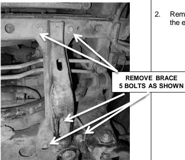
2. Remove the front left brace located between the engine & radiator cross members.
