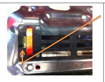
23. If factory stone shield is fitted, attach warning label as shown.
