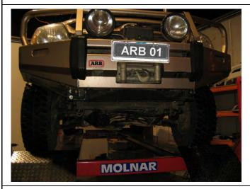
1. Remove stone shield or under vehicle protection (UVP).
