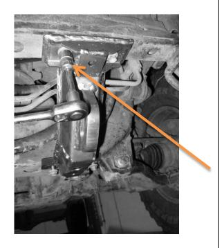
5. Fit M10x1.25x30 mm bolt, spring & flat washer to fasten the recovery point to the chassis (5 bolts) finger tight only.
