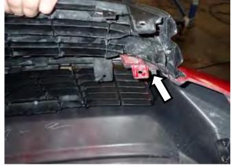
18. Remove grille from bumper by carefully releasing locking tabs whilst removing.
