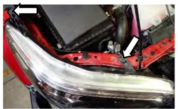
19. With grille and bumper removed, remove LH and RH headlight retaining fasteners to allow headlight to be moved forward giving access to indicator/headlight wiring.
