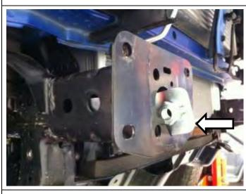
42. Insert 2 x M12x1.75 nut plate into RHS chassis rail as shown.
