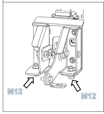
51. Loosely install 2 x M12 x 1.75 x 35 bolts, spring washers and flat washers through lower mount and chassis support brackets into M12 x 1.75 flange nuts.
