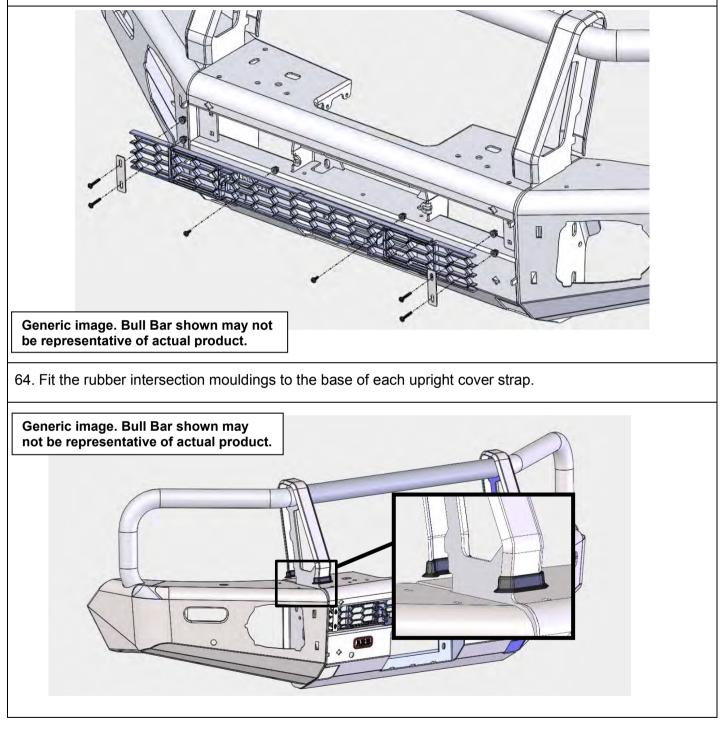
65. From the rear of the bar, slide the rear buffer sections under the rubber mouldings.
