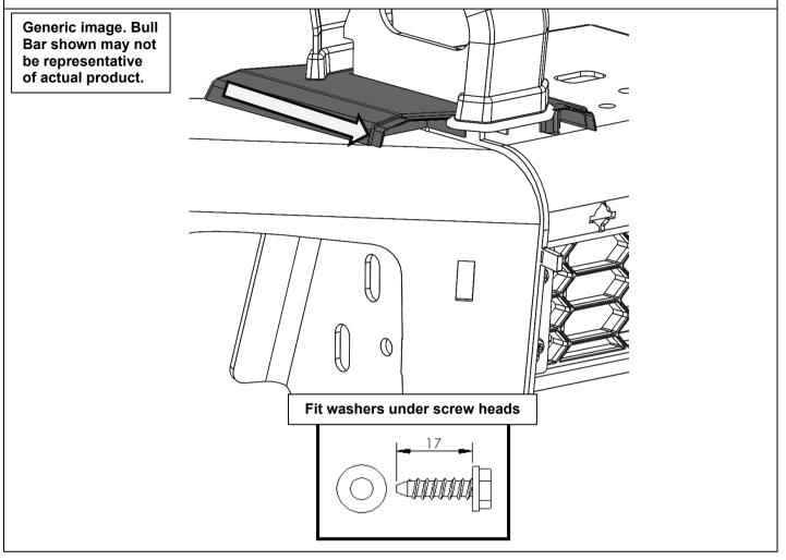
66. By aligning the front buffer with the tongue of the rear buffer, attach the front buffers to the front face of the bar. Ensure each buffer sits flat against the face of bar and is keyed into the top section of the rear buffer.
