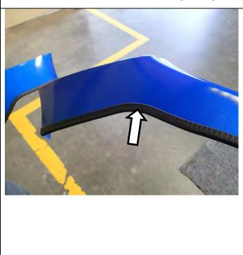
37. Apply bumper trim pinch weld to both RH and LH sides. Use the 480mm length on the outer edge and the 88mm on the inner.
