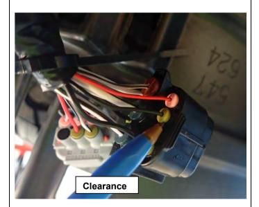
62. On the Driver's side Remove OE wiring loom bracket as shown with Phillips head screw driver. Detach plugs from bracket and discard bracket, it will not be reused. Unplug both the black and grey plugs
