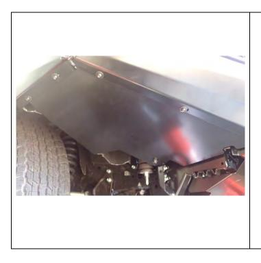
88. Trim the fender liner end flush with the splash panel face as shown. Then tuck the remaining wheel liner inside the wing panel return.
