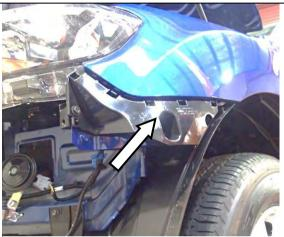
14. Remove screws retaining RH & LH bumper retention blocks to vehicle and remove the retention blocks from both sides and set aside.
