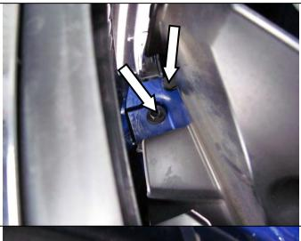
64. Undo and remove the screws and plastic clips behind the grille near the lower inner edge of the head lights.
