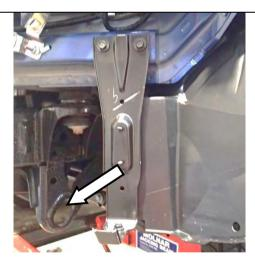
15. Remove and discard the inner guard support brackets from both sides of the vehicle.
