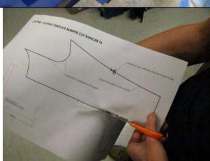
108. Using scissors carefully cut out the supplied paper template 3787985 for Ranger PX 2011-15.
