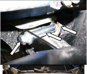
140. Secure the rear of the chassis braces to the chassis using 2 x M10 x 80 bolts, 2 x M10 spring washers and 2 x M10 flat washers through 2 x crush tubes into the nut plate assemblies on each side of the vehicle. Leave loose at this stage.
