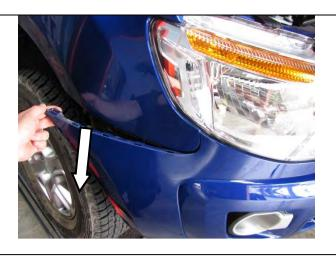
66. Starting on the RH side of the vehicle, carefully pull the rear most corner away from the vehicle un-clipping the bumper. With the assistance of another person remove the bumper from the vehicle and place in a safe place where it will not be damaged. Disconnect the sensor attached to the bumper and allow it to hang loose. If fog lights are fitted they will need to be disconnected.
