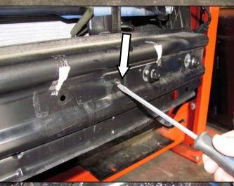
11. Use a screw driver to push the 2 x plastic clips inward from the front cross beam.Do not remove the clips as they will be used later.
