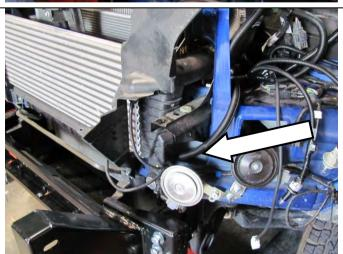
93. Route the remainder of the loom across the front of the vehicle along the cross beam that runs below the intercooler as shown.
