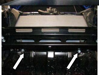
141. Re fit the OE stone shield to the bracket fitted in step 81 using 2 x M10 SEMS bolts and 2 x M10 flange nuts.
