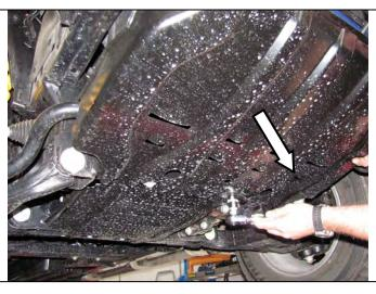
70. Remove the factory under panel and place in a safe place. Do not completely remove the rear bolts. Leave loose.
