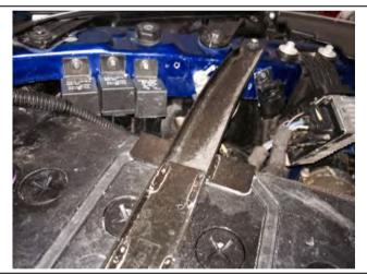
86. Using the tek-screws provided, attach the 3 relays to the panel directly behind the LH head light as shown.
