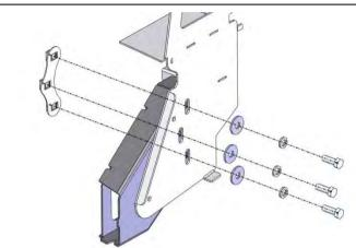
149. Attach the bar to the mount bracket using 6 x M12 bolts, 6 x M12 spring washers and 6 x large diameter M12 flat washers, into the nut plates which are placed inside the box upright sections of the mount bracket. Leave loose at this stage.
