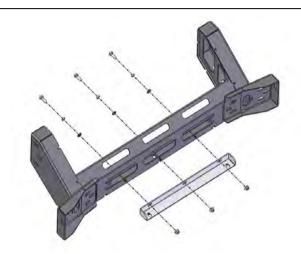
139. Attach the OE stone shield bracket to the chassis mount using 3 X M8 x 25 black bolts, 3 X M8 black flat washers, 3 X M8 black spring washers and 3 X M8 flange nuts. Leave loose at this stage.
