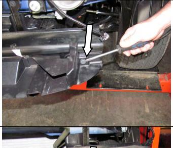
10. Remove the plastic panel attached to the front cross beam by removing the plastic clips. Discard the panel.
