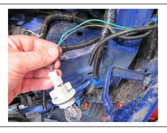
88. On each side of the vehicle, carefully cut back the protective tubing from the turn light globes wiring being careful not to damage the wires inside.
