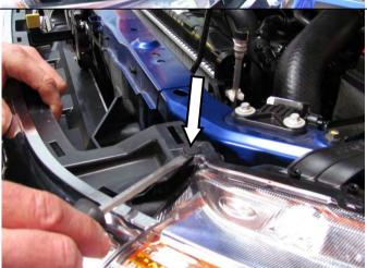
61. Remove the plastic clips from the top / rear corners of the grille. Place clips in a safe place.
