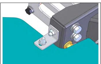
163. On each side of the bar attach the under wing panel to the mount bracket with the wing panel bracket using 2 M8 hex bolts, 2 M8 spring washers, 2 M8 flat washers and 2 M8 flange nuts.
