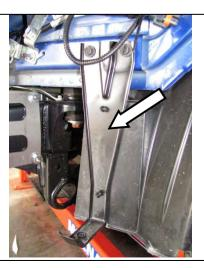
73. Remove and discard the inner guard support brackets from both sides of the vehicle.
