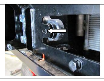
142. Using the original plastic clips re-fit the factory air deflector to the 2 holes in the mount bracket
