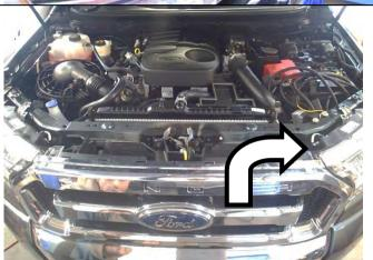
2. Remove the screws and retaining clips used to retain grille.
