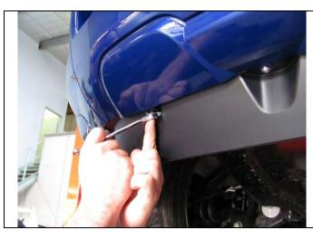
63. Remove all the fasteners securing the bottom of the bumper to the vehicle.
