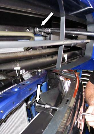
65. Using a socket extension, remove the screws holding the inner grille air deflectors to the vehicle. Place in a safe place.
