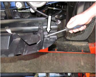
67. Remove the plastic panel attached to the front cross beam by removing the plastic clips. Discard the panel.
