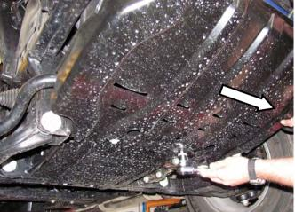
12. Remove the factory under panel and place in a safe place. **Do not completely remove the rear bolts. Leave loose.**
