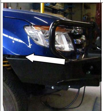
150. Position the bar so that it is level and there is a gap between the top face of the wings and the bottom edge of the guards, for 2011-15 PX of 18-22mm and 15ON PX2 25-30mm. The wing tips are to be aligned with the edge of the wheel arch.
