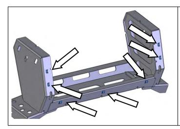
138. Fit 7 X M8 cage nuts into the mount bracket from the inside.
