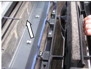
71. Carefully unclip the grille from the bumper and place in a safe place.
