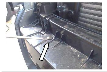
8. Carefully remove all clips used to retain bumper to crash beam.
