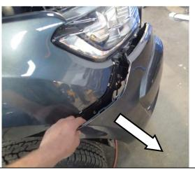
9. Starting on the RH side of the vehicle, carefully pull the rear most corner away from the vehicle un-clipping the bumper. With the assistance of another person remove the bumper from the vehicle and place in a safe place where it will not be damaged. Disconnect the sensor attached to the bumper and allow it to hang loose. If fog lights are fitted they will need to be disconnected.
