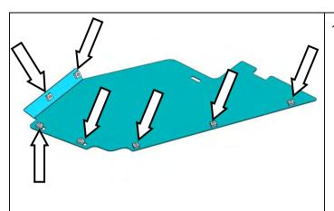
160. Fit 7 x M6 cage nuts to each of the under wing panels as shown.
