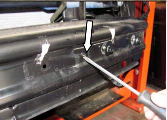
68. Use a screw driver to push the 2 plastic clips inward from the front cross beam. Do not remove the clips as they will be used later.
