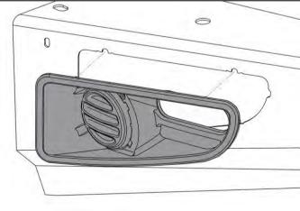
158. Assemble and install combination light surrounds (p/n 3163015) as per instructions no. 3786421 supplied with surround kit. Note: Optional fog lamps can be installed at this point as per fitting instruction no. 3783315 supplied with fog lamp kit no. 6821201.
