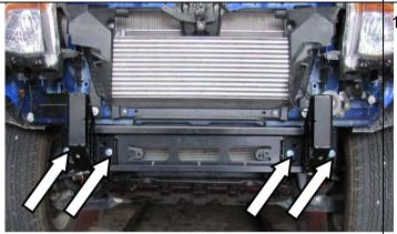
33. Attach the mount bracket to the chassis end plates using 4 X M10 SEMS bolts into the captive nuts. Leave loose at this stage.
