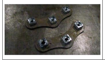
147. Fit 3 x M12 cage nuts to each of the cage nut plates.
