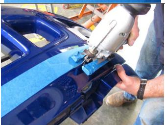
107. Using a jig saw or similar, carefully cut along the line made in the previous step.
