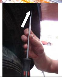
62. Remove all the bumper fasteners along the inside edge of the wheel arches.
