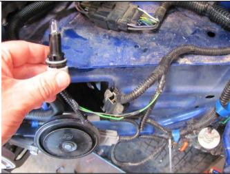
89. On the left side of the vehicle, carefully cut back the protective tubing from the clearance light globe wiring being careful not to damage the wires inside.
