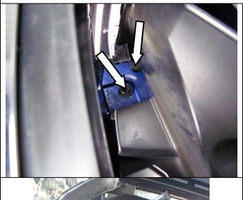
5. Undo and remove the screws and plastic clips behind the grille near the lower inner edge of the head lights.
