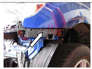
72. Remove the RH and LH bumper retention blocks from either side of the vehicle and place in a safe place.
