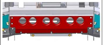
175. Attach the centre stone shield to the mount bracket using 7 M8 hex bolts, 7 M8 spring washers and 7 M8 flat washers into the cage nuts fitted in step 139.
