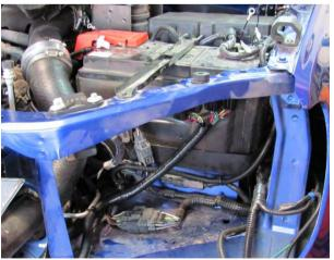
87. Route the battery positive and the battery negative wires to the relevant sides of the vehicles battery. Do not attach at this stage.
