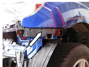
Remove the RH and LH bumper retention blocks from either side of the vehicle and place in a safe place.
