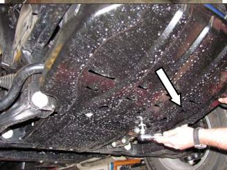
11. Remove the factory under panel and place in a safe place.
