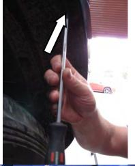
3. Remove all the bumper fasteners along the inside edge of the wheel arches.
