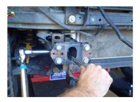
72. Using a spanner to hold the M16 flange bolt, torque the M16 flange nut.
