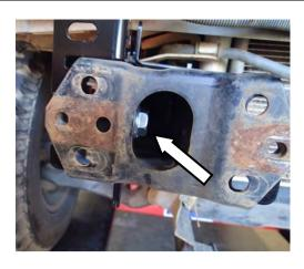
69. Fit the M16 x 35 flange bolt through the front access cut out of the front flange of the chassis.
