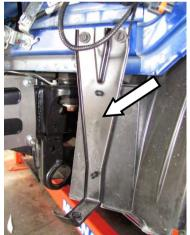
14. Remove and discard the inner guard support brackets from both sides of the vehicle.
