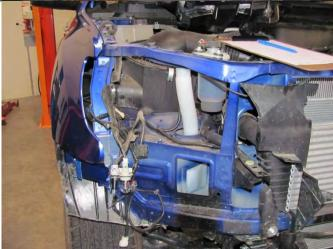
27. Following fitting instructions 3789197 supplied in kit 6821287; attach the LED combination lamp looms (also supplied in same kit).
