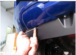
4. Remove all the fasteners securing the bottom of the bumper to the vehicle.
