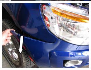
7. Starting on the RH side of the vehicle, carefully pull the rear most corner away from the vehicle un-clipping the bumper. With the assistance of another person remove the bumper from the vehicle and place in a safe place where it will not be damaged. Disconnect the sensor attached to the bumper and allow it to hang loose. If fog lights are fitted they will need to be disconnected.
