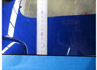
Note: The line should end up being 90mm below the edge of the bumper that mates with the vehicles guard.
