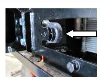
88. Using the original plastic clips re-fit the factory air deflector to the 2 x holes in the mount bracket.
