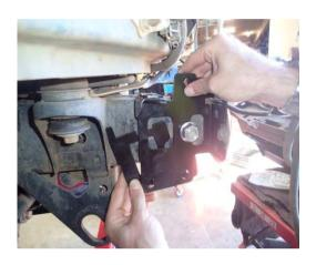
70. Loosely position the outer bracket brace with the packer to the chassis rail. Apply LOCTITE 243 then fit the M16 flange nut to hold it in place. Ensure that the front edge is pushed forward to the chassis flange.
