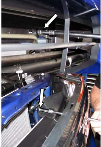
6. Using a socket extension, remove the screws holding the inner grille air deflectors to the vehicle. Place in a safe place.
