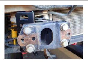
71. Fit 4 x M12 x 35 bolts, 4 x M12 flat washers, 4 x M12 Flange nuts.
