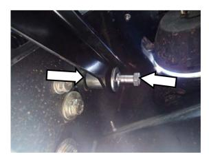
111. Fit the 35mm wide spacer and the M12 x 1.75 x 80 bolt, M12 washer and M12 spring washer.
