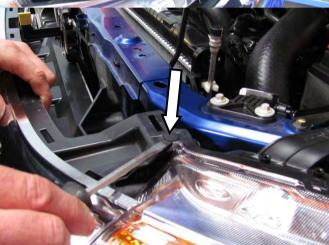
2. Remove the plastic clips from the top / rear corners of the grille. Place clips in a safe place.
