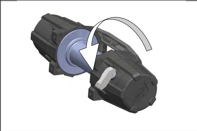
2. Use above chart as a guide to positioning the clutch handle. Generally they are in the 72° or 144° anti-clockwise position. Remove the gearbox fasteners and rotate the gearbox to the required position. **DO NOT REMOVE GEARBOX COMPLETELY.** Tighten when done.
