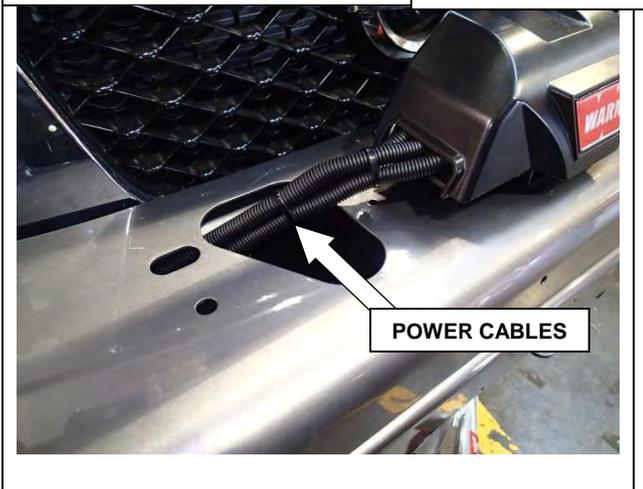
9. Place the sections of 13mm dia split tubing on the three black cables coming out of the control box.
