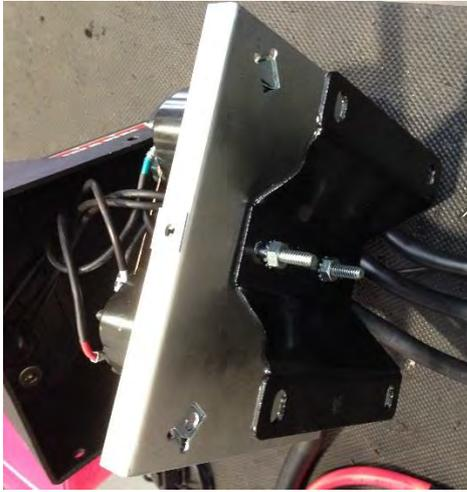
1. Attach control box to control box bracket using fasteners removed from control box in earlier step, so that the top face of the bracket is flush with the bottom surface of the control box.
