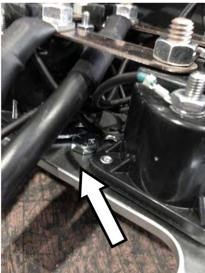
1. Undo 2 X supplied M6 nuts from underside of control box. To do so, top of M6 bolts located on the inner side of the box will need to be held in place.
