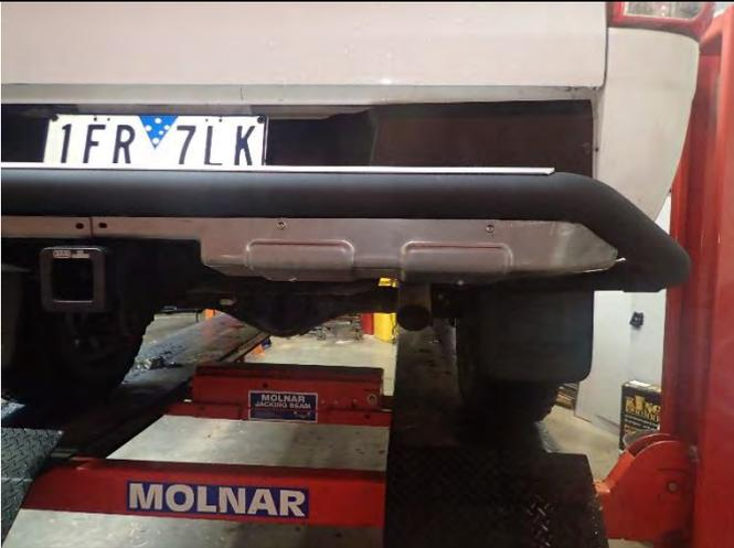
60. Attach the diffuser panels to the RSTB using 10 M6x16 button head screws and M6 stainless flat washers.
