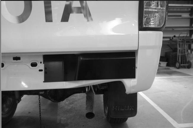
33. Temporarily fasten beaver panel to rear of tub and align upper edge of beaver panel so it is parallel with tailgate lower edge.
