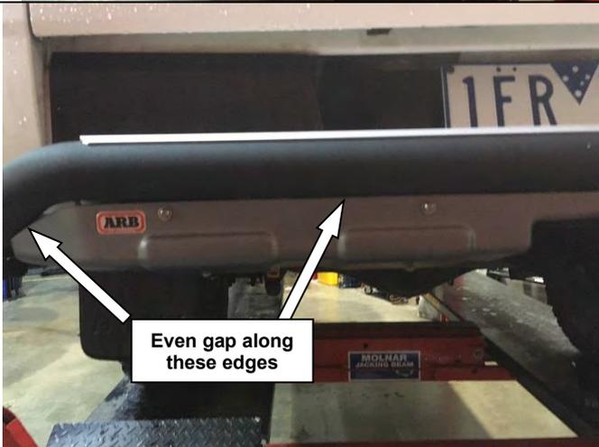
61. Position each diffuser panel so there is an even gap between the panel and the RSTB tube. Tighten fasteners to the specified torque.
