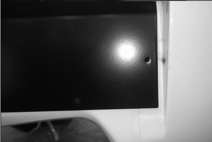
34. When the alignment is achieved drill  $\text{Ø}6.5\text{mm}$  hole through tub face. Remove temporary fasteners holding beaver panel in place. De-bur the hole to remove all sharp edges.
