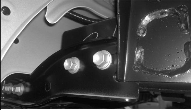
2. If fitted, remove the 2 M8 bolts from the headlight levelling sensor guard and then remove the M8 bolt from the cable clamp
