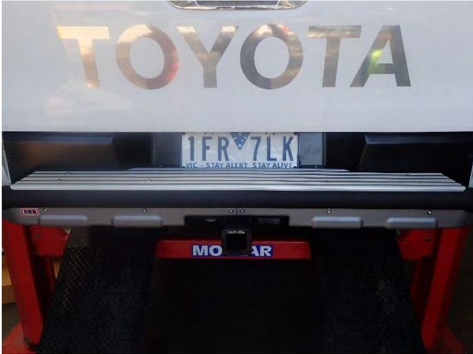
62. Attach the step plate extrusion to the RSTB using 8 M6x1.0x16 button head screws. Proceed to tighten fasteners installed in step 61
