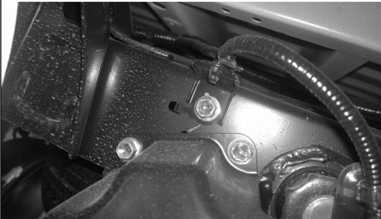
3. Remove the spare wheel from beneath the tub using the wheel nut wrench and jack handle pieces supplied with the vehicle. Insert as shown through the access slot above the number plate position and rotate counter-clockwise to release the wheel.
