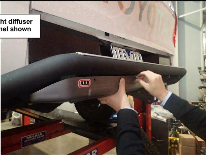
59. Position the diffuser panels on either side of the receiver tube as shown.
