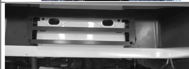
45. Fix the license plate assembly to the beaver panel using 4 M6x1.0x16 button head screws, 8 M6 flat washers (black), and 4 M6 nyloc nuts as shown.
