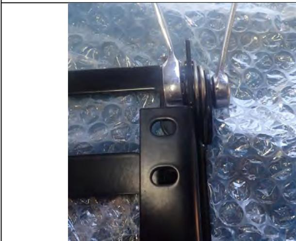
44. Tighten the M6 bolts on both LH and RH brackets enough so the brackets can be rotated by hand but not freely by themselves.
