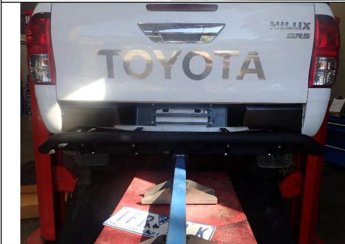
48. With the assistance of other people or a lifting device, lift the RSTB up beneath the chassis rails aligning the threaded holes in the side of the chassis with those in the vertical surfaces of the RSTB.
