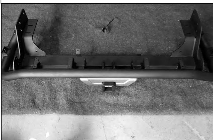
39. Rotate the RSTB 90° so it is now resting flat on the ground as shown.
