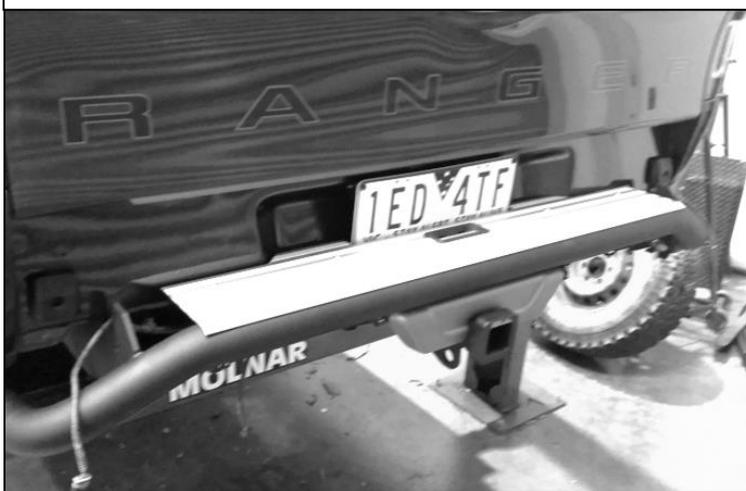
79. Attach the step plate extrusion to the RSTB using 8 M6x16 button head screws taking care not to damage the LED lamp wire.
