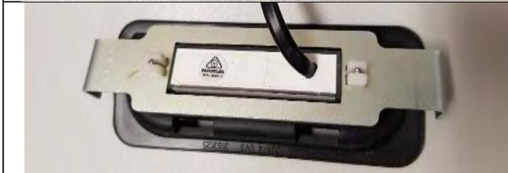
69. Fit the clear plastic plugs supplied in the lamp kit to the LED lamp above the screws.
