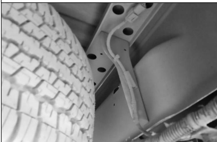
80. Route the LED lamp loom through the RSTB to its fastening point identified in Step 1 and connect to the existing connector.
