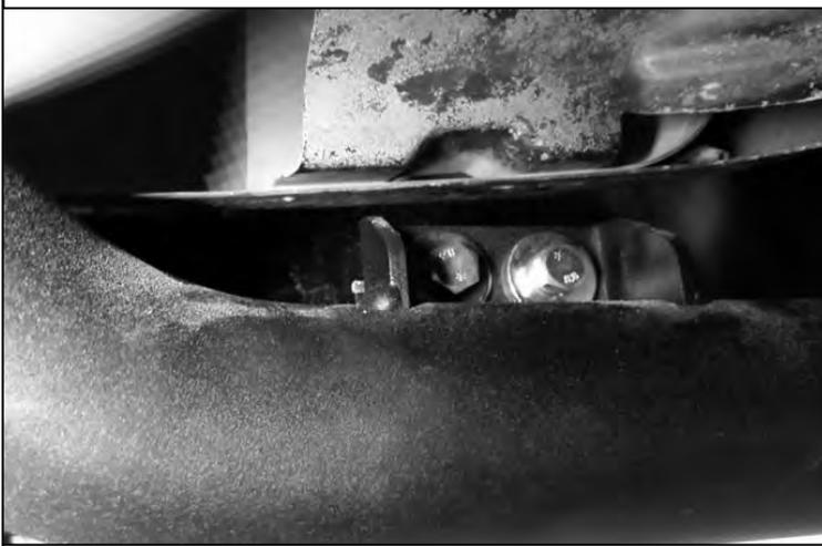
102. Fix the middle bracket of each Ranger wing to the RSTB tube using 2 M8x1.25x25 hex head bolts, 2 M8 spring washers, 2 M8 flat washers and the wing double nut plate already fitted. Leave bolts finger tight at this stage.
