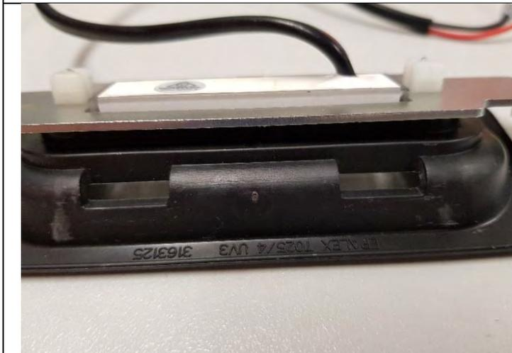
67. **Remove the foam ring from the LED lamp and discard.**
