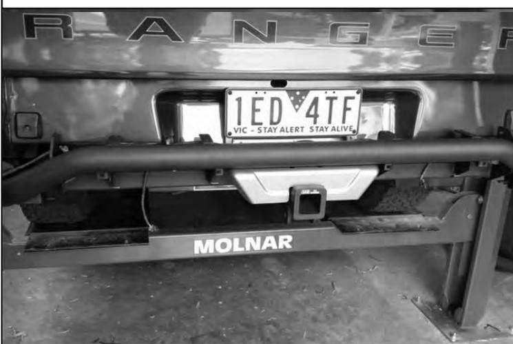
63. Tidy and fasten all wiring using cable ties and the slots in the RSTB brackets, as well as existing fastening locations.
