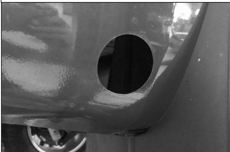
88. De-bur each hole to remove sharp edges.
