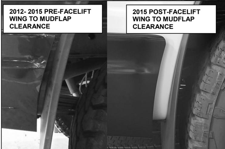
104. Position each Ranger wing so they there is an even gap to the mud flap as shown.
