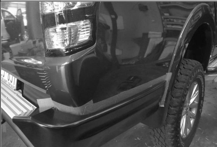
71. With the assistance of other people or a lifting device, position the Triton wing next to the rear side vehicle panels. Take care not to damage the vehicle when positioning the Triton wing.
