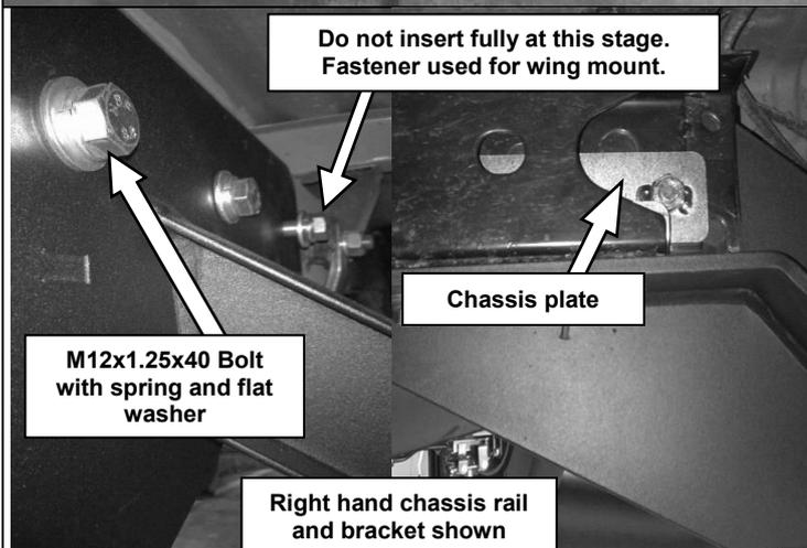
52. Fix the vertical plates of the RSTB to the chassis plate from fitting kit in each chassis rail using 3 M12x1.25x40 (fine pitch) hex head bolts, 3 M12 spring washers and 3 M12 flat washers per chassis rail. Leave finger tight at this stage as shown.
