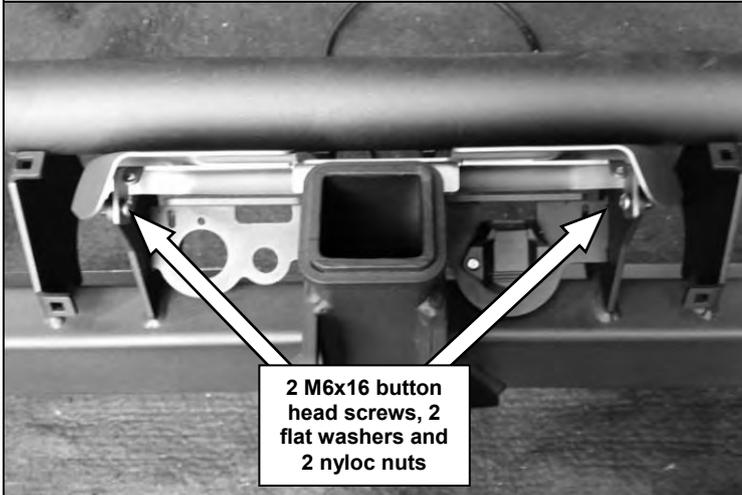
29. Attach the lift up panel to the pivot plates on the RSTB using 2 M6x16 button head screws, 4 M6 flat washers and 2 M6 nyloc nuts.
