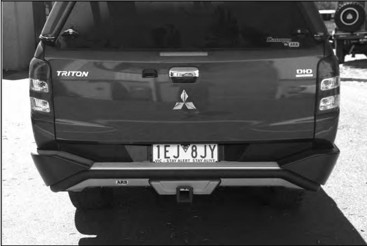
83. Reattach the spare wheel beneath the vehicle. Return licence plate to upright position and tighten up licence plate bolts that were previously loosened in step 87
