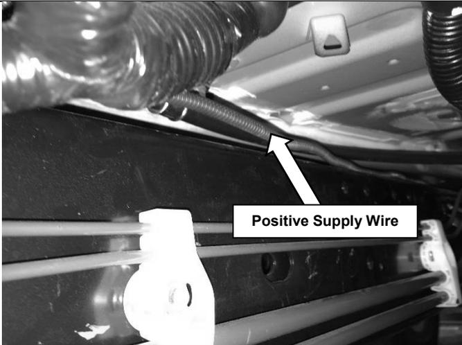
16. Route the positive supply wire to the front of the vehicle following the existing vehicle harness along the left chassis rail.
