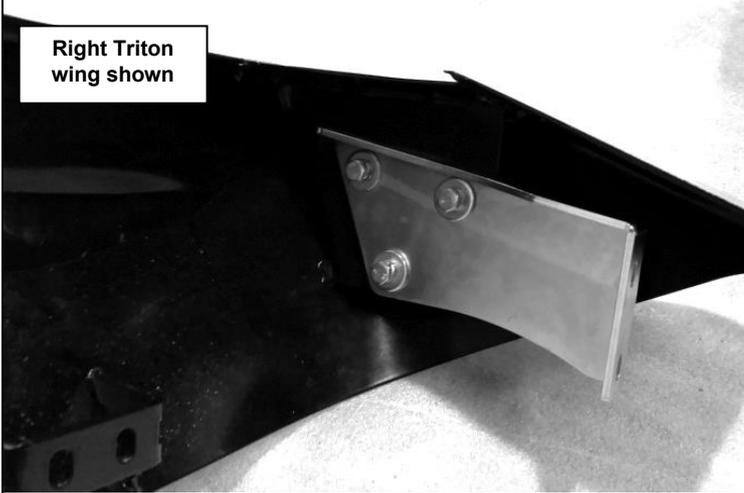
66. Fix a wing mount bracket to each Triton wing using 3 M8x1.25x25 hex head bolts, 3 spring washers, 3 flat washers and a wing triple nut plate. Orientate each bracket as shown. Leave bolts finger tight at this stage
