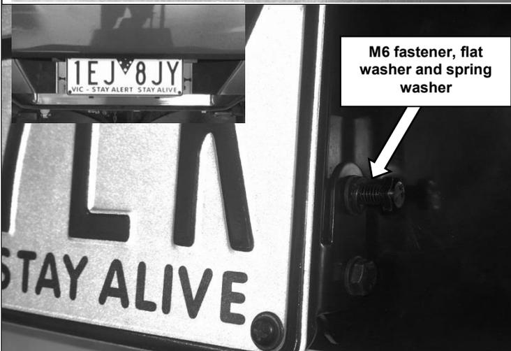
49. Using 4 screws supplied fasten licence plate to frame.
