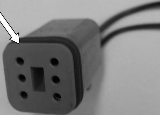
10. Insert the white blank pin into position 6 as shown in the previous step.
