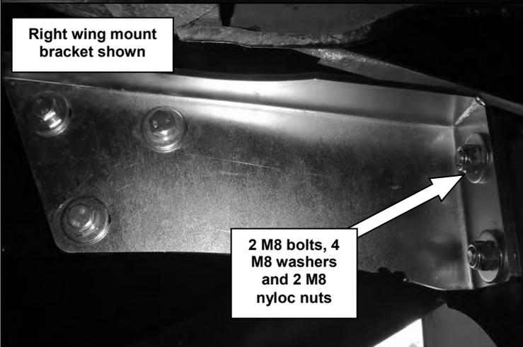
73. Fix the wing mount bracket of each Triton wing to the RSTB using 2 M8x1.25x25hex head bolts, 4 M8 flat washers and 2 M8 nyloc nuts. Do not fully tighten at this stage.
