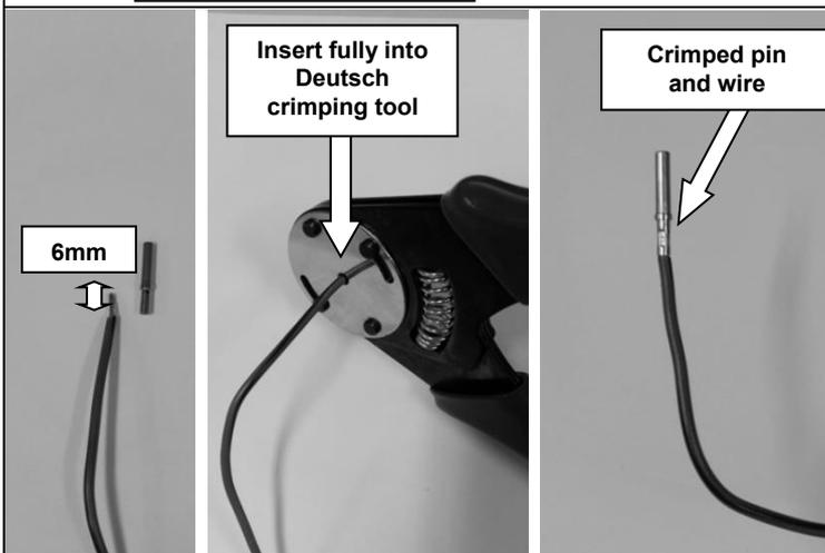
6. Remove 6mm of the plastic insulation coating from the end of each newly cut wire.
