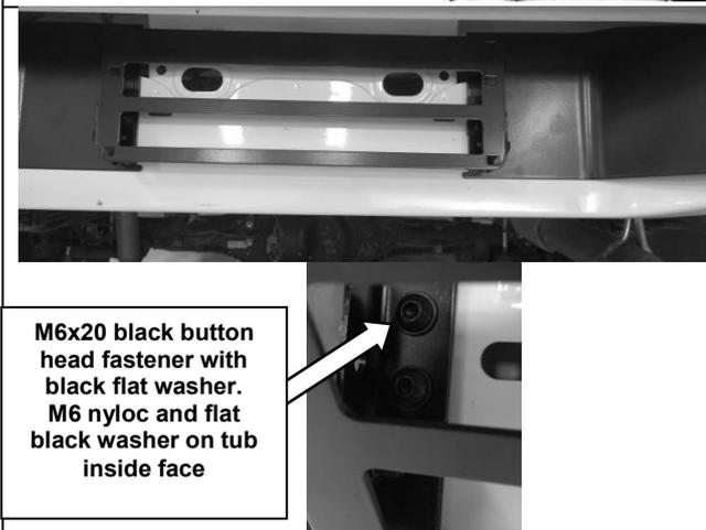
M6x20 black button head fastener with black flat washer. M6 nyloc and flat black washer on tub inside face
