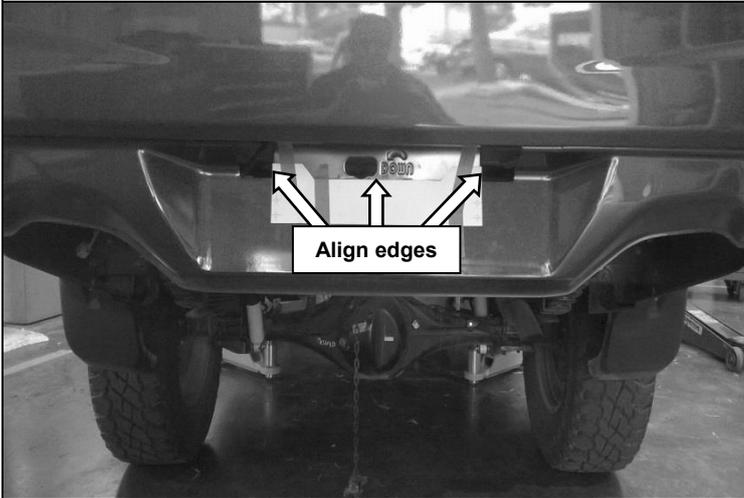
36. Place the number plate drilling template on the rear panel of the tub as shown. When aligned use masking tape to hold in place
