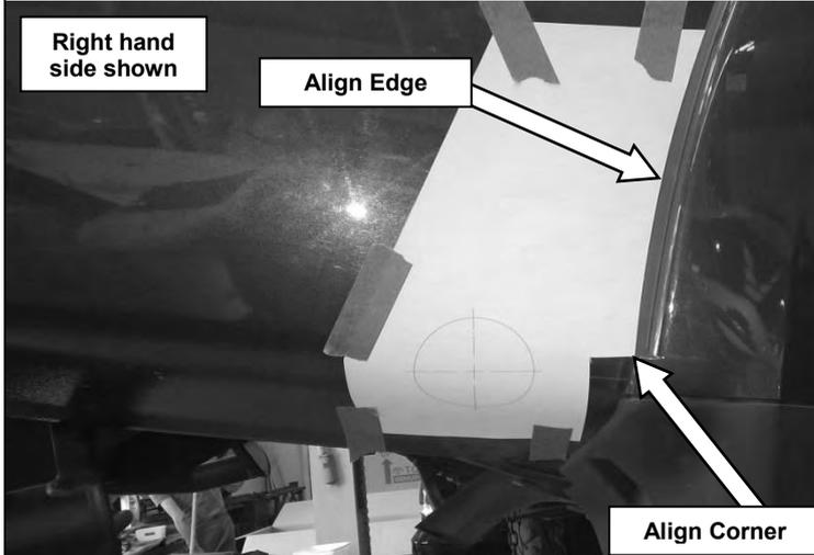
60. Place the cutting template on the right hand rear side panel of the tub aligning it with the flare edge of and step of flare as shown. Use masking tape to hold in place.
