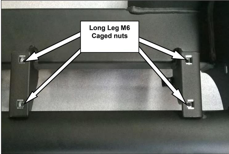
34. Fit 8 long-leg M6 caged nuts to the RSTB. Fit 4 caged nuts to the right side as shown and 4 cage nuts to the left hand side
