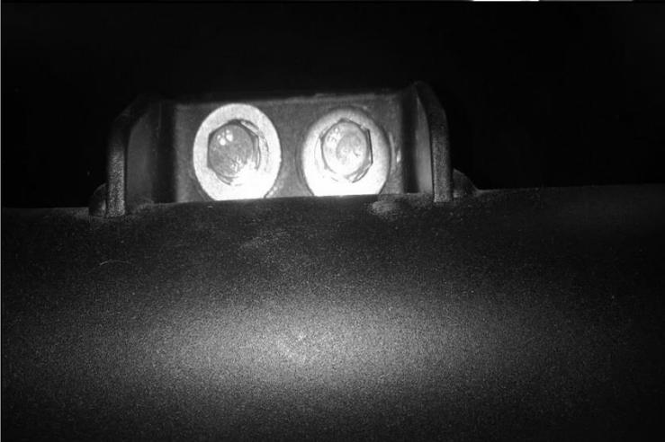
74. Fix the middle bracket of each Triton wing to the RSTB tube using 2 M8x1.25x25hex head bolts, 2 M8 spring washers, 2 M8 flat washers and the wing double nut plate already fitted. Leave bolts finger tight at this stage.
