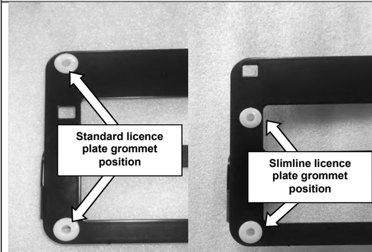
48. Insert 4 plastic grommets into number plate frame to suit licence plate size
