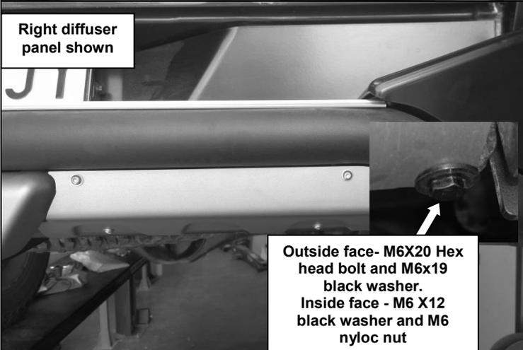
80. Attach the diffuser panels to the RSTB using 8 M6x16 button head screws and M6 stainless flat washers. For the outer most screw on each panel, retain using 2 M6X20 hex head bolts, M6x19 black washer and M6x12 black washer and M6 nyloc nut as shown.
