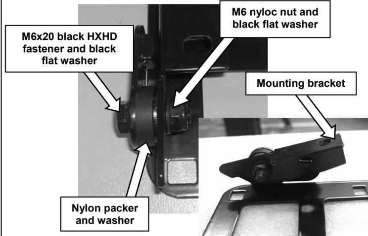
44. Assemble license plate bracket as shown taking note of mounting bracket orientation. Repeat step for opposite side of license plate bracket.
