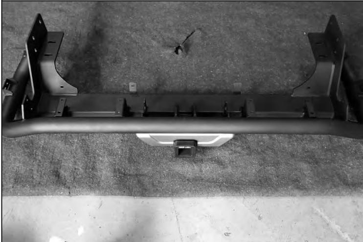
31. Rotate the RSTB 90° so it is now resting flat on the ground as shown.
