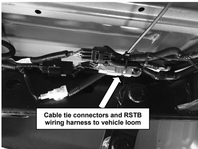
19. Connect the RSTB wiring harness to the 2 male 6-pin connectors.
