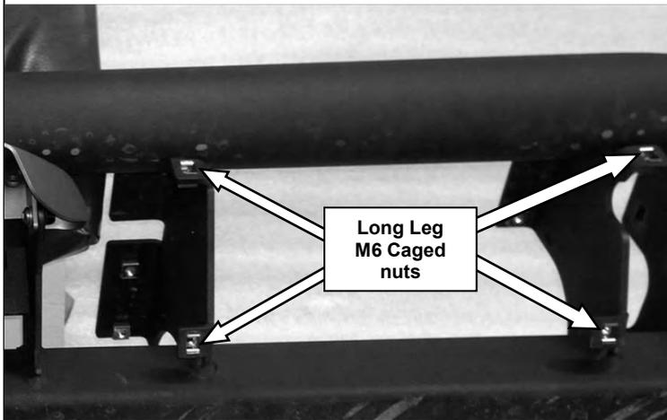
35. Rotate and support the RSTB and fit 8 long-leg M6 caged nuts. Fit 4 caged nuts to the right side as shown and 4 cage nuts to the left hand side
