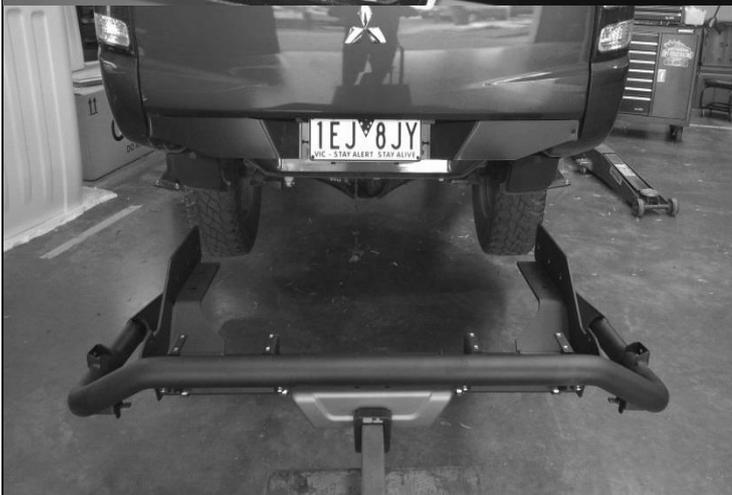
51. With the assistance of other people or a lifting device, lift the RSTB up beneath the chassis rails, aligning the threaded holes in the side of the chassis with those in the vertical surfaces of the RSTB.
