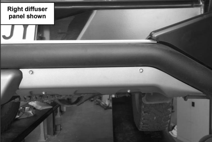
79. Position the diffuser panels on either side of the lift up panel as shown.
