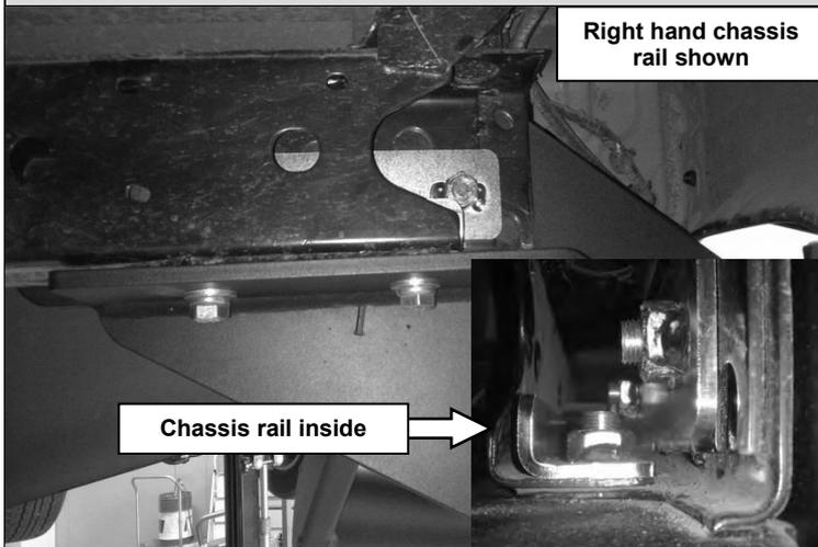
53. Insert folded chassis plate from fitting kit as shown inside chassis and fasten the remaining horizontal mount points using 2 M12x1.25x40 (fine pitch) hex head bolts, 2 M12 spring washers and 2 M12 flat washers
