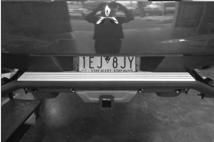
59. Attach the step plate extrusion to the RSTB using 8 M6x16 button head screws taking.
