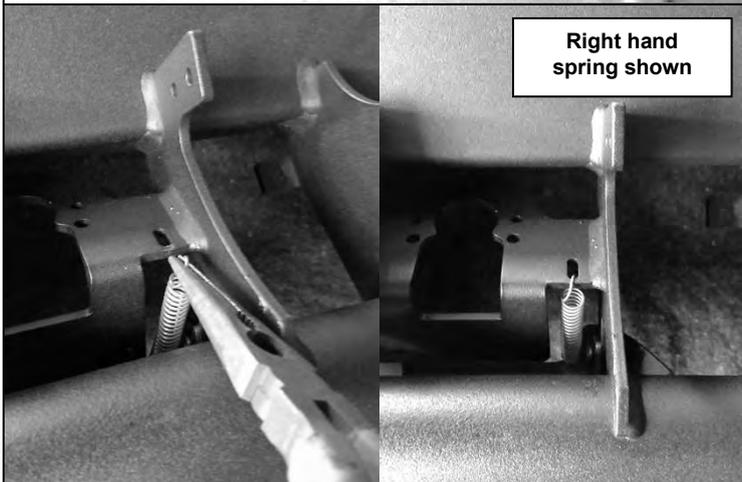
33. Using pliers, stretch the free end of each spring up to the bracket on the RSTB as shown.
