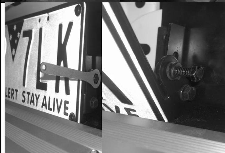
82. Using 10mm spanner provided release licence plate retaining bolt on both sides sufficiently to allow licence plate to pivot down
