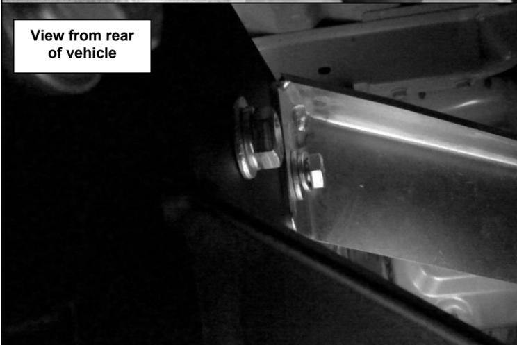
68. Position the right hand wing mount strut under the tub and fix to the vertical plate of the RSTB.
