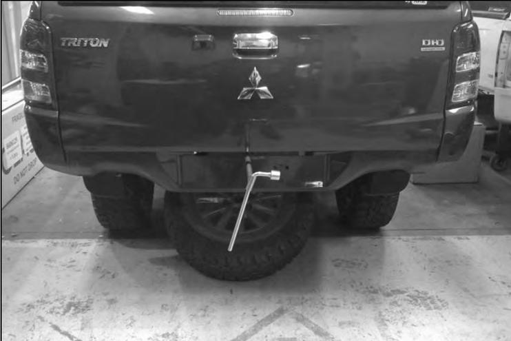
3. Remove the spare wheel from beneath the tub using the wheel nut wrench and jack handle pieces supplied with the vehicle. Insert as shown through the access slot above the number plate position and rotate counter-clockwise to release the wheel.
