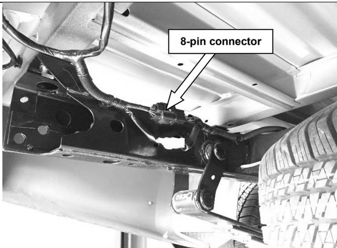
4. Locate the 8-pin connector on the left hand chassis rail behind cross member as shown. Disconnect connector and remove tape if present and expose 200mm of the following coloured wires from the PVC/corrugated tubing:
