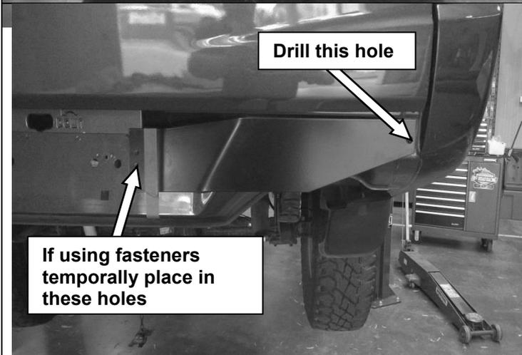
38. Temporarily fasten beaver panel to rear of tub with either tape or fasteners and align upper edge of beaver panel so it is parallel with tailgate lower edge
