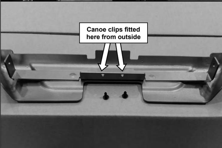
28. Fit 2 plastic canoe clips to the lift up panel using the holes as shown.
