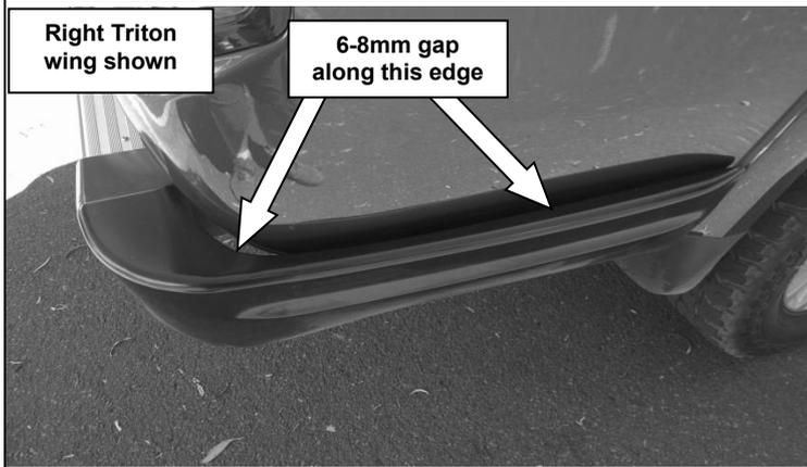
75. Position each Triton wing so there is an even 6-8mm gap to the side vehicle panels.
