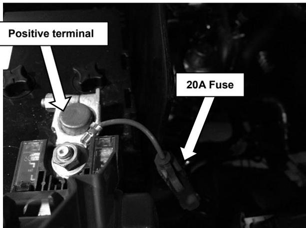
17. Continue routing the positive supply wire through the engine bay to the battery.
