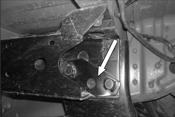
2. Remove bolt plate from inside of chassis rail from each side and discard as shown and remove bumper bar
