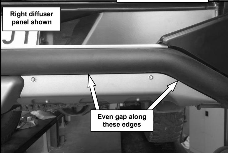
81. Position each diffuser panel so there is an even gap between the panel and the RSTB tube. Tighten fasteners to the specified torque.
