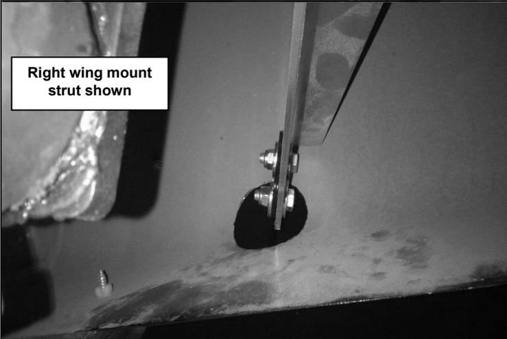
72. Pass the front bracket of each Triton wing through the  $\text{\O}70\text{mm}$  hole in the tub and fasten to the wing mount strut using 2 M8x1.25x25hex head bolts, 4 M8 flat washers and 2 M8 nyloc nuts. Do not fully tighten at this stage.
