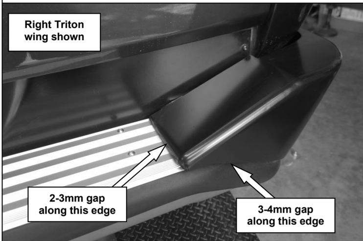
77. Position each Triton wing so they sit evenly on the step plate extrusion and there is an even gap to the tube as shown.
