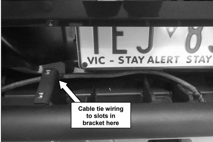
57. Tidy and fasten all wiring using cable ties and the slots in the RSTB brackets, as well as existing fastening locations.
