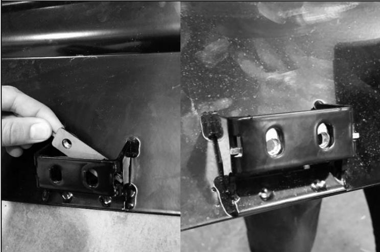
67. Place a wing double nut plate inside the middle bracket of each Triton wing as shown.
