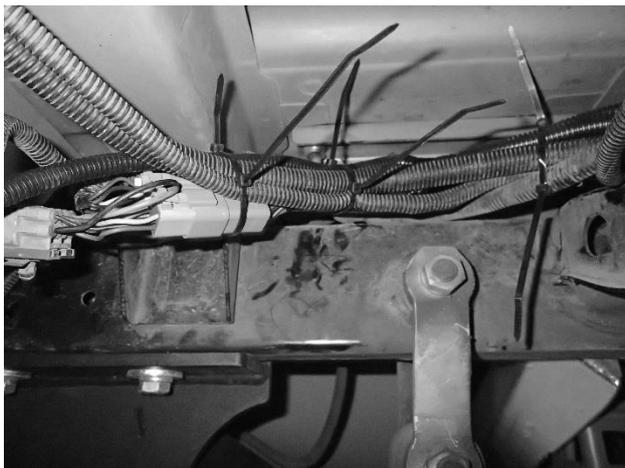
24. Tidy and fasten all wiring using the cable ties provided.
