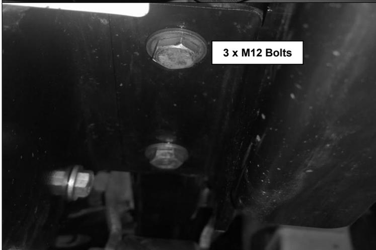
4. Remove the bumper bar from the vehicle by removing M12 bolts from each chassis rail as shown.
