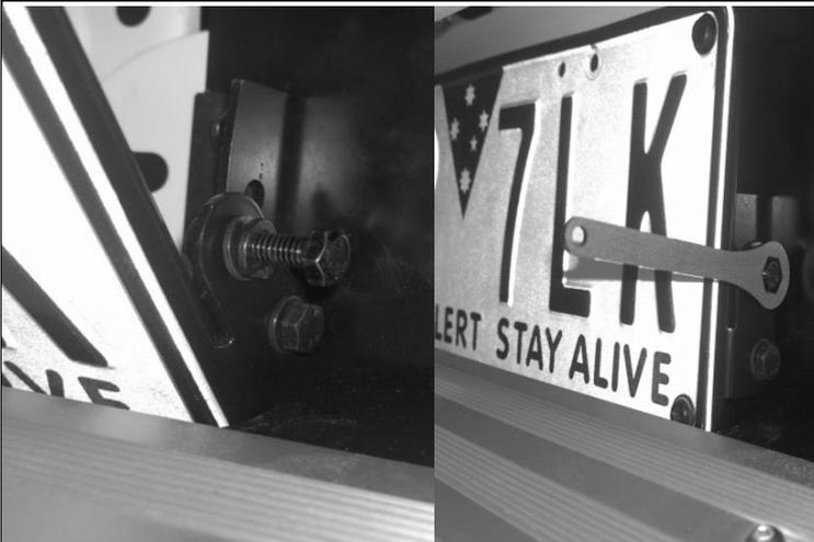
89. Using the 10mm spanner provided tighten the licence plate retaining bolt on both sides to secure the licence plate in an upright position
