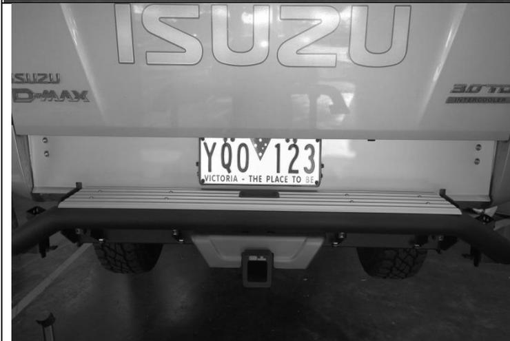
63. Attach the step plate extrusion to the RSTB using 8 M6x1.0x16 button head screws taking care not to damage the LED lamp wire.
