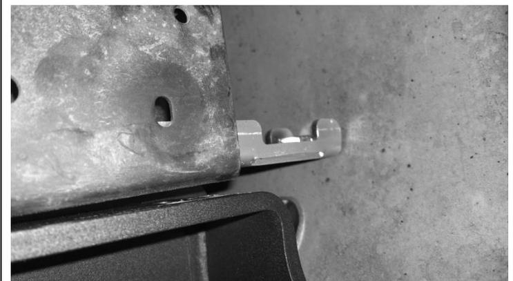
50. Insert the folded chassis plates in chassis and fasten the remaining horizontal mount points using 2 M12x1.25x40 (fine pitch) hex head bolts, 2 M12 spring washers and 2 M12 flat washers. Leave finger tight at this stage.
