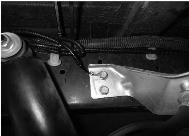
23. Connect the ground wire of the RSTB harness to the bolt on the inside of the rear chassis rail as shown.
