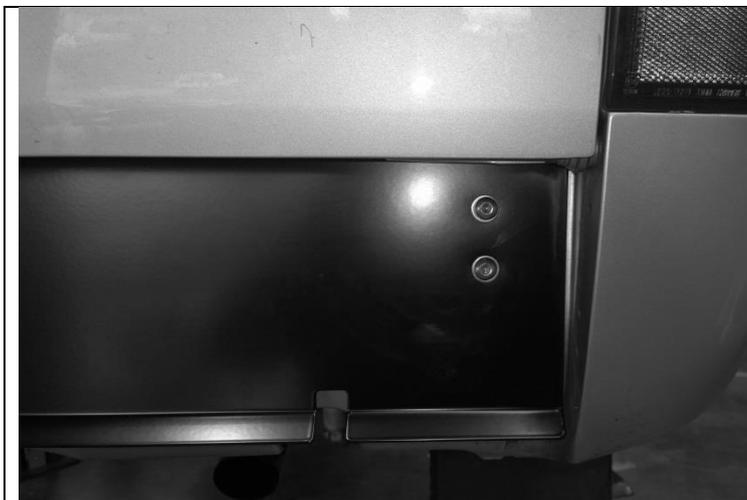
43. Continue to fix the beaver panel assembly to the vehicle using, 4 M8x1.25x20 button head screws, 4 M6x1.0x16 button head screws, 4 M8 flat washers (SS) and 4 M6 nyloc nuts.
