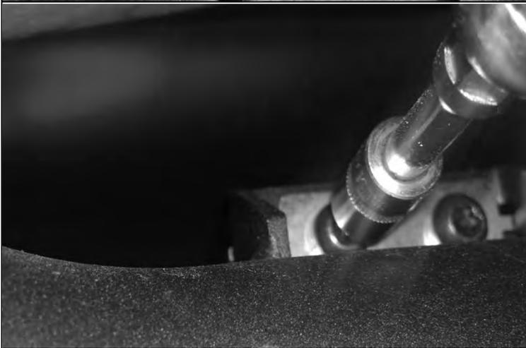
80. Fix the middle mount bracket of each DMAX wing to the RSTB using 2 M8x1.25x25 torx head bolts, 2 M8 spring washers and retainer plate as shown. Do not fully tighten at this stage.
