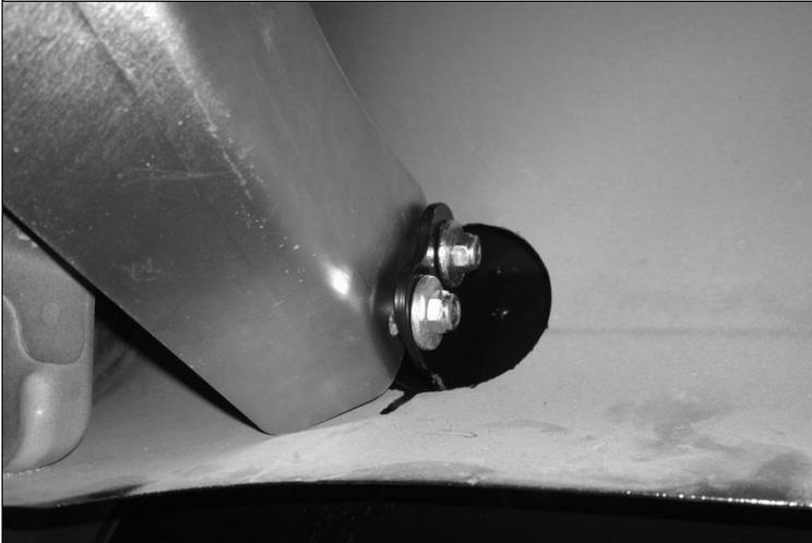
78. Pass the front bracket of each DMAX wing through the  $\text{\O}70\text{mm}$  hole in the tub and fasten to the wing mount strut using 2 M8x1.25x25 hex head bolts, 4 M8 flat washers and 2 M8 nyloc nuts. Leave bolts finger tight at this stage.
