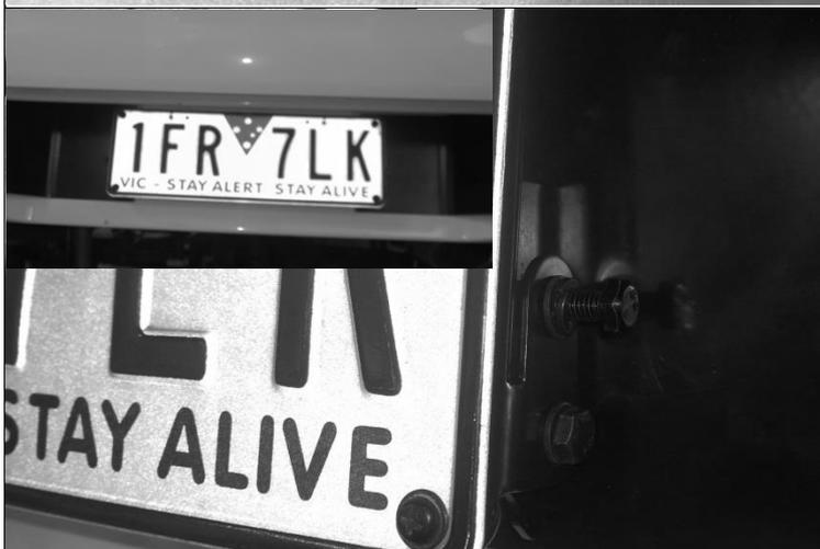
47. Using 4 screws supplied fasten licence plate to frame.
