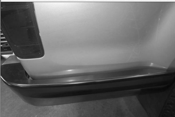
81. Position each DMAX wing so there is an even 6-8mm gap to the side vehicle panels.
