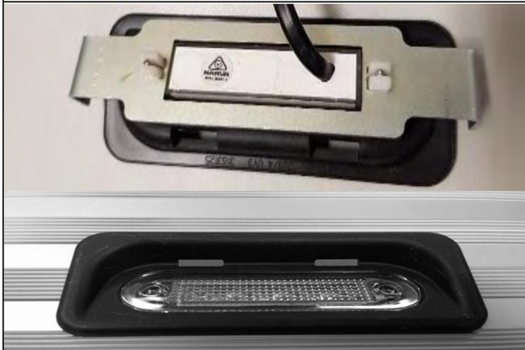
57. Fit the clear plastic plugs supplied in the lamp kit to the LED lamp above the screws.
