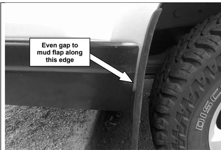
82. Position each DMAX wing so they there is an even gap to the mud flap as shown.
