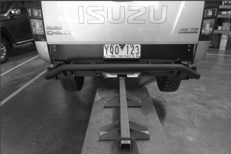
48. With the assistance of other people or a lifting device, lift the RSTB up beneath the chassis rails aligning the threaded holes in the side of the chassis with those in the vertical surfaces of the RSTB.
