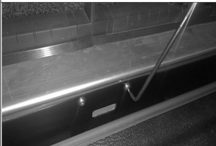
42. Fix the beaver panel assembly to the vehicle using, 2 M8x1.25x20 button head screws, 2 M6x1.0x16 button head screws, 2 M8 flat washers (SS) as shown.
