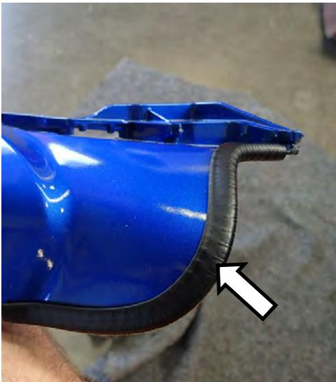
34. Apply bumper trim pinch weld to both RH and LH sides along the full length of the cut edge. Carefully trim off any excess length.
