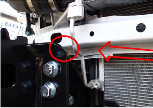
48. Loosely install 2 x M12 x 35 bolts, spring washers and flat washers through lower mount and chassis support brackets into M12 flange nuts. **Note: Starting with the M10 bolts installed from the front of the mount, tighten all fasteners enough to eliminate any play in mount or support brackets but to still allow for adjustment of bullbar.**
