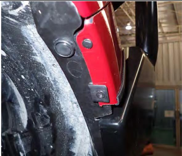
92. Re-Install clip as shown and re-install clip scrivet.
