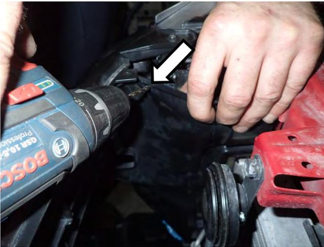
36. Using a 5mm – 6mm drill bit carefully drill a hole through the upper front corners of the air deflector panels. (RH shown).
