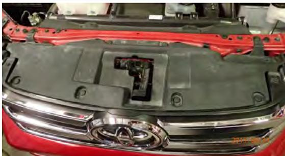
94. Re-install upper radiator cover panel and fasten using 8 x OE scrivets.
