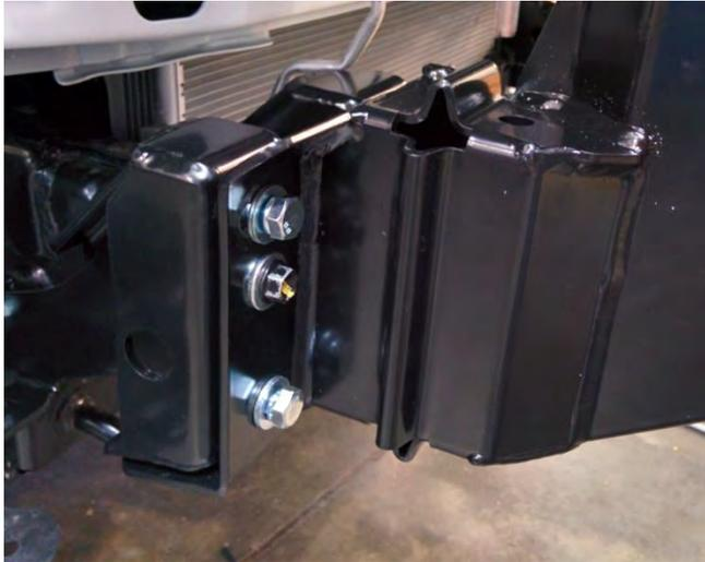
71. Adjust position of bar left/right until it's sitting central to body, then tighten all inner fasteners joining mount assembly to chassis brackets (2 x M10 and 1 x M10 OE bolts each side).
