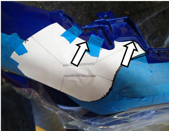
26. Position Template 3789446 onto RHS of bumper. Align the profiled shape at the top corner of the template with the corresponding profiled area on the bumper whilst aligning with the ridge on the bumper as specified on template.
