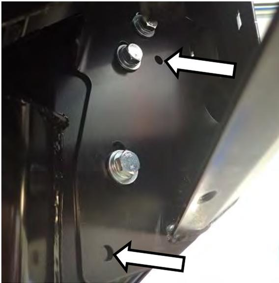
75. Drill 4 x Ø10mm holes (2 per side) through mount assembly using existing holes in bull bar as guide.
