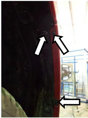
4. Remove all fasteners and scrivets retaining bumper along inside edge of wheel arches – (Right hand side shown).
