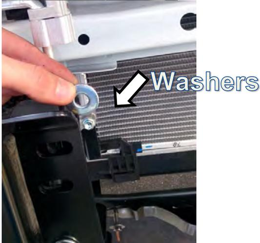
44. On both RH And LH installation it is extremely important that 1 x M10 x 25 x 3mm flat washer per hole is installed on the upper holes between the support brackets and the mount when offering the mount up to the chassis flange. The upper M10 bolts as installed in Step 47 should pass through the mount, spacer washers and the support brackets.
