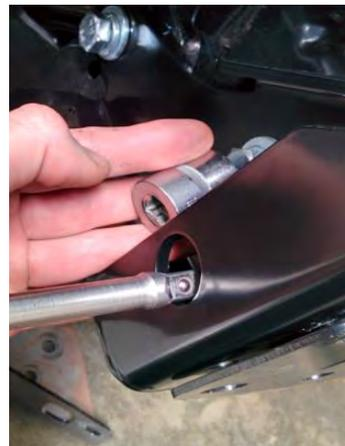
**NOTE: IF USING A LARGE SIZE SOCKET, IT MAY BE NECESSARY TO PLACE THE SOCKET OVER THE FRONT BOLT BEFORE INSERTING AN EXTENSION THROUGH THE HOLE IN THE FLANGE.**
