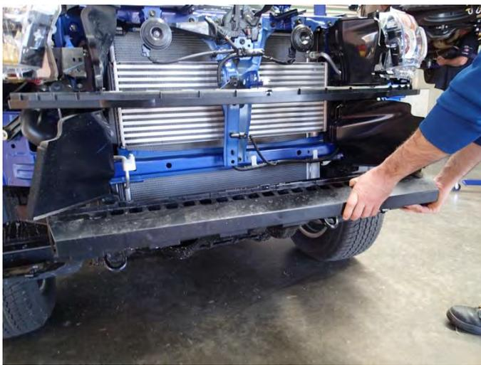
11. Remove plastic lower crush absorber from vehicle and discard.
