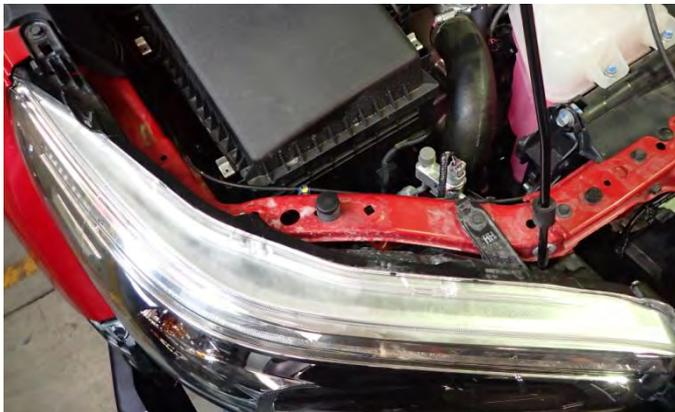
21. Re-install LH and RH headlights using fasteners retained from step 19.
