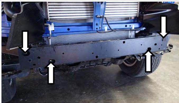
14. Remove 2 x M10 bolts on both sides (4 total) fixing crash beam to chassis and remove crash beam.
