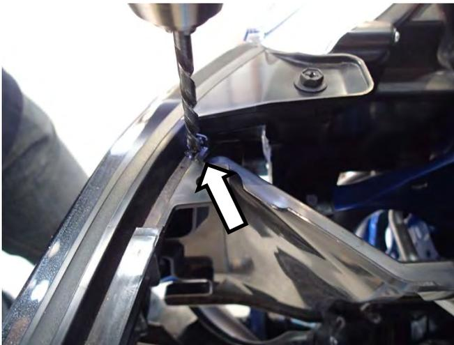
37. Using a 5mm – 6mm drill bit carefully drill a hole through the top face of the grille panel in line with the air deflector panel. (RH shown).
