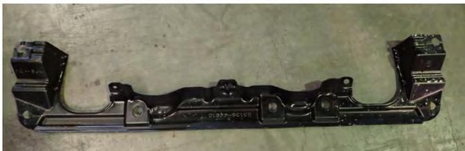
7. Remove dressing piece from underside of bumper and discard.
