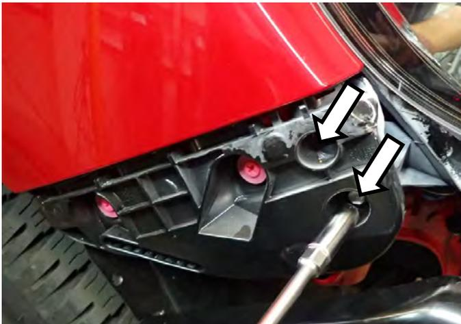
19. With grille and bumper removed, remove LH and RH headlight retaining fasteners to allow headlight to be moved forward giving access to indicator/headlight wiring.
