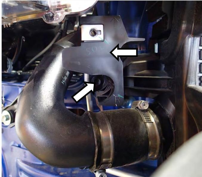
13. Remove M8 fastener from upper crush panel support brackets. Remove support brackets from vehicle and discard. (Right hand side shown).
