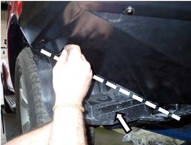
83. Mark lines onto the OEM inner guards (LH & RH) using lower edge of wing under panels as guide ensuring enough guard remains so that it may be neatly tucked/secured behind wing under panel lip.
