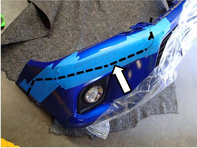
32. Carefully cut bumper along marked lines using a hack saw or jig saw and remove all masking tape.
