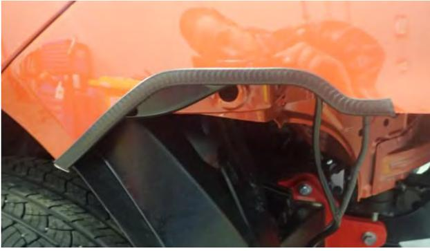
35. Fit Pinch weld to RH side along the full length of the cut edge. Carefully trim off any excess length and use remainder for other side.
