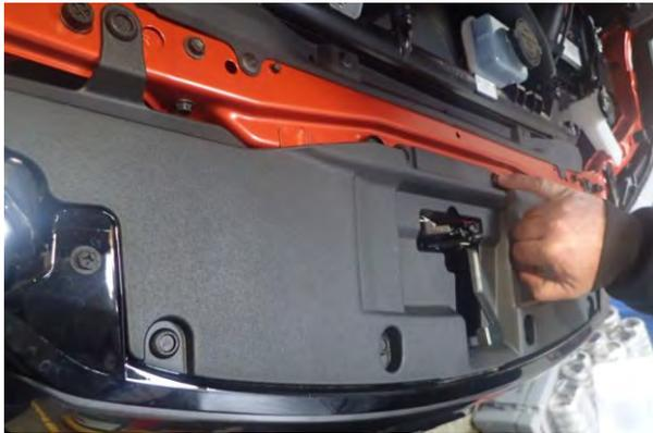
87. Re-install upper radiator cover panel and fasten using 8 x OE scrivenets.
