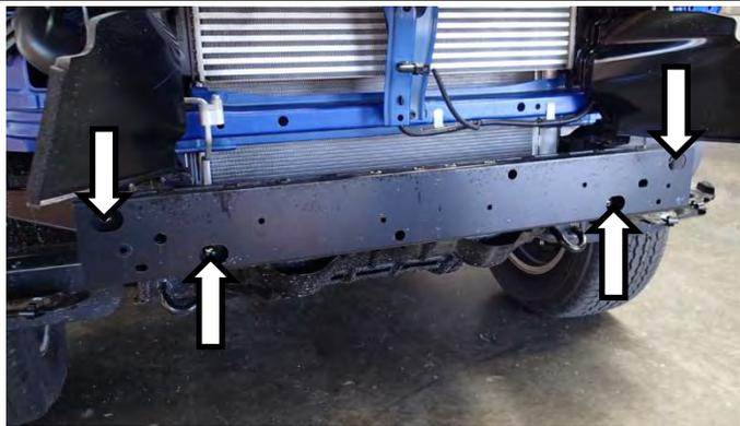
15. Remove 2 x M10 bolts on both sides (4 total) fixing crash beam to chassis and remove crash beam.
