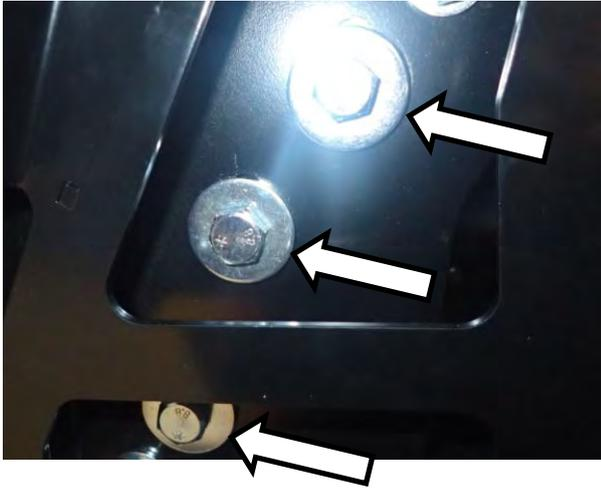
67. Loosely fasten bar to mounts using 6 x M12 x 1.75x35mm bolts, 6 x M12 flat washers (4mm thick) and 6 X M12 flange nuts.
