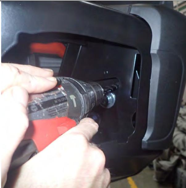
72. Drill 4 x Ø10mm holes (2 per side) through mount assembly using existing holes in bull bar as guide.
