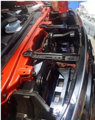
3. Remove upper grille retaining screws (4).
