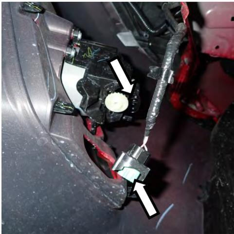
11. Disconnect fog light wiring – (Right Hand side shown).
