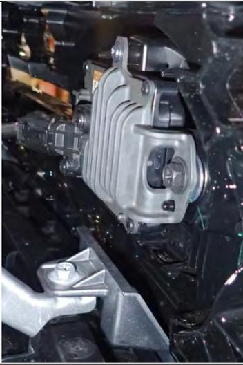
9. If vehicle is equipped with adaptive cruise control, unplug radar (located behind Toyota badge)
