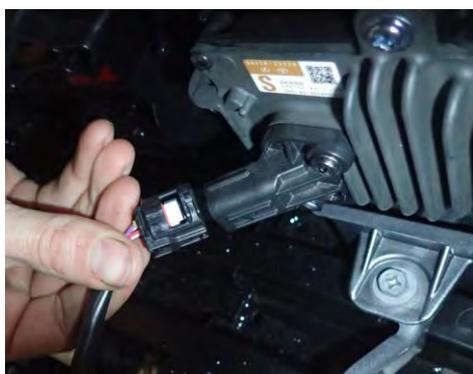
34. If vehicle is equipped with adaptive cruise control, reconnect radar.
