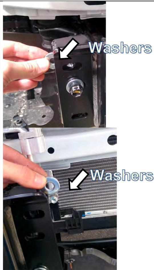
41. On both RH and LH installation it is extremely important that 1 x M10 x 25 x 3mm flat washer per hole is installed on the upper holes between the support brackets and the mount when offering the mount up to the chassis flange. The upper M10 bolts as installed in step below should pass through the mount, spacer washers and the support brackets.
