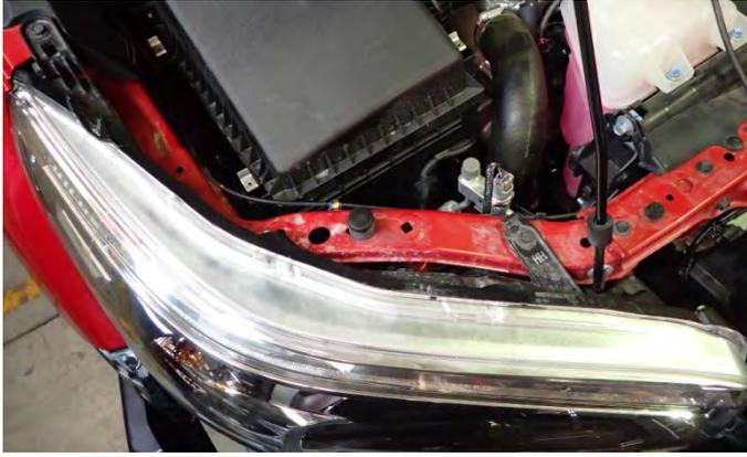
21. Re-install LH and RH headlights using original fasteners.
