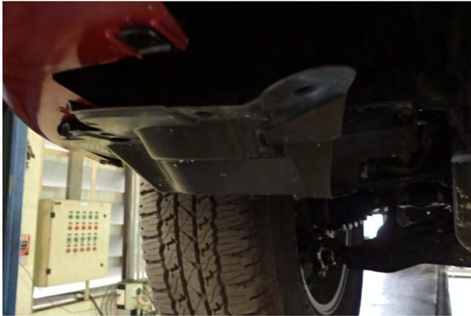
10. Ensure inner guards are unclipped from front bumper.
