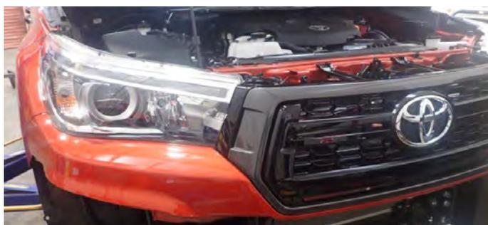
33. Re-install trimmed bumper and grille using OE fasteners removed in previous steps.
