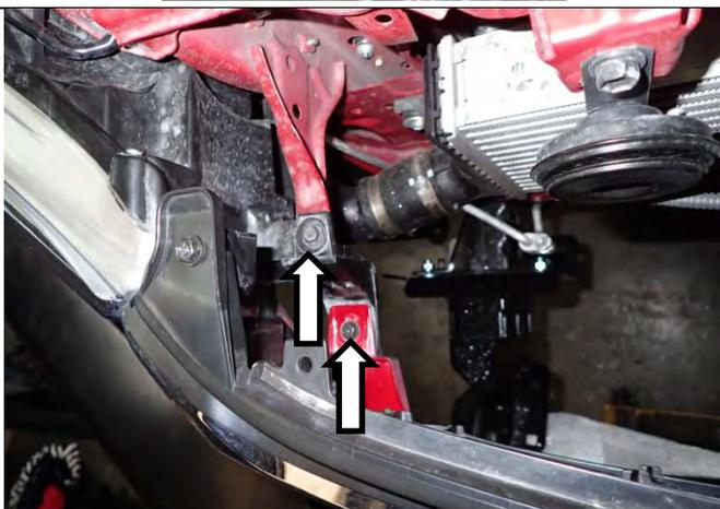
4. Remove lower grille retaining screws – (Right hand side shown).
