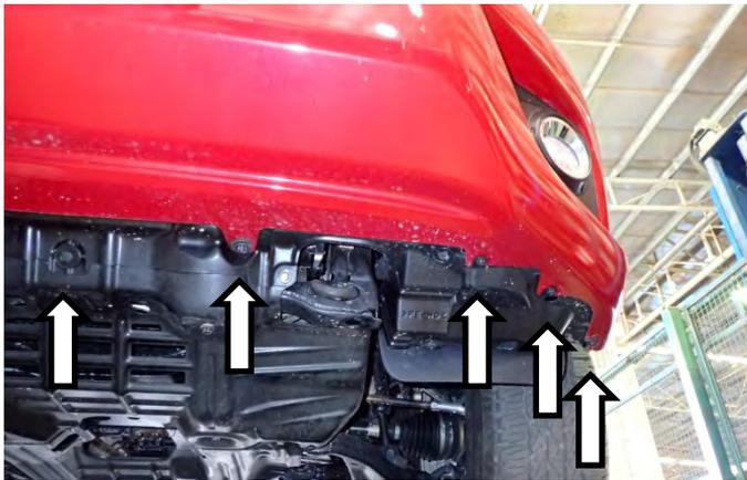
7. Remove all fasteners and scrivets retaining bumper along lower lip – (Left Hand side shown).
