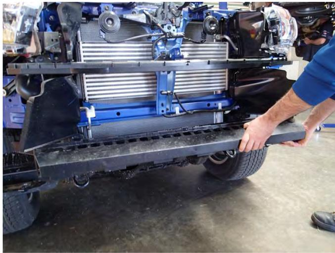
14. Remove plastic lower crush absorber from vehicle and discard.
