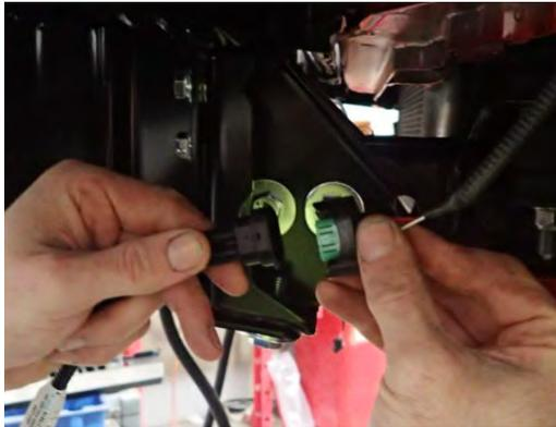
77. Using extension harnesses supplied, connect fog lights to vehicle loom.
