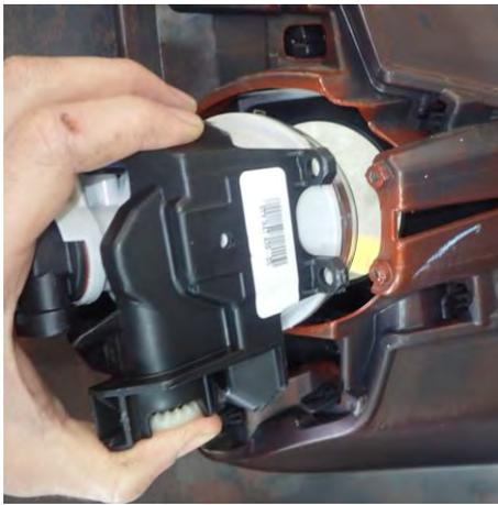
13. If fitted, remove fog lights from bumper and set aside for reuse in bull bar.
