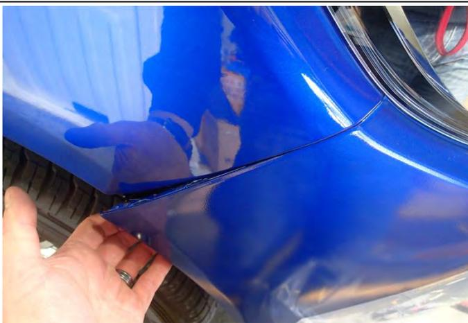
12. Remove registration plate and set aside, then carefully remove bumper from vehicle by pulling on each side of the bumper near the wheel arches and working your way towards the centre.
