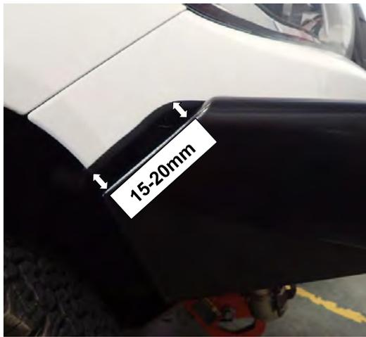
70. Position the bar so that it is level with the bumper cut profile as shown and there is an even gap of 15-20mm between the wing edge and bumper cut trim.
