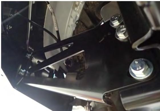
78. Remove all outer fasteners joining mount assembly to chassis brackets (2 x M10 and 1 x M10 OE bolts each side). Assemble and install wing braces using 2 x M10 SEMS bolts and flange nuts on each brace.
