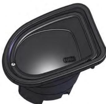
85. Assemble and install combination light surrounds (p/n 3163082) as per instructions no. 3789190 supplied with surround kit. Note: Optional fog lamps can be installed at this point as per fitting instruction supplied with fog lamp kit no. 3500590
