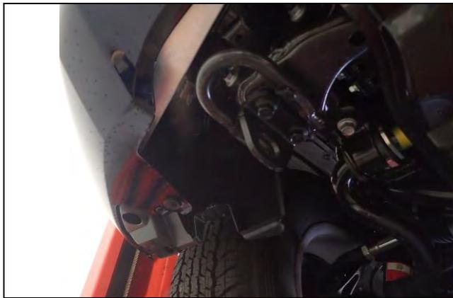
9. Remove right and left splash guards located at the recovery hooks.
