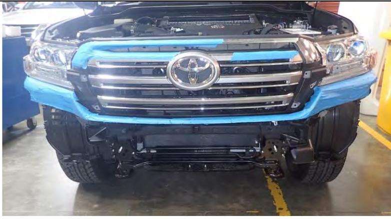
35. Fit the cut bumper and grille and secure. as shown
