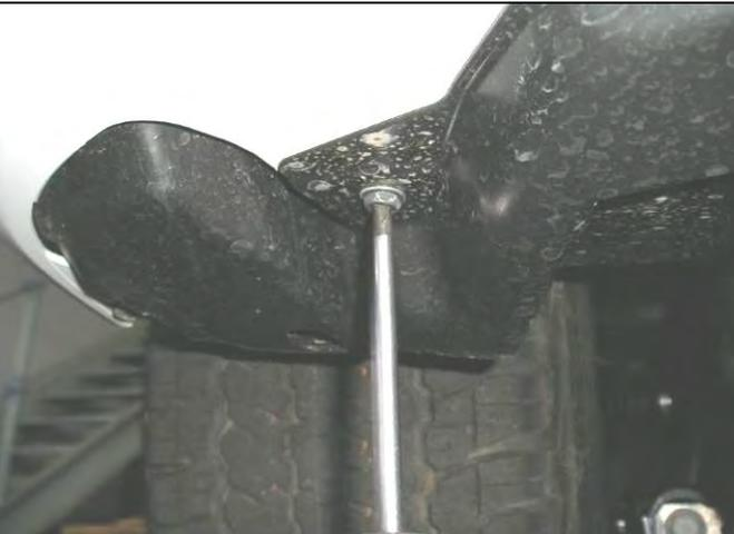
3. Remove lower trim panel sets each side which attach to bumper and engine protective plate area then set aside, they will not be reused.
