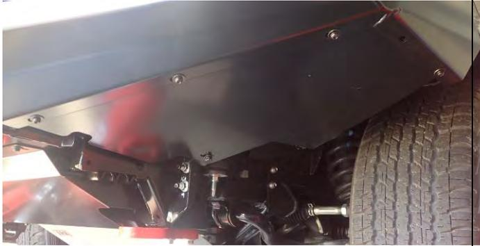
93. Fit 5 x M6 cage nuts to each wing splash panel as shown on *inside* faces.
