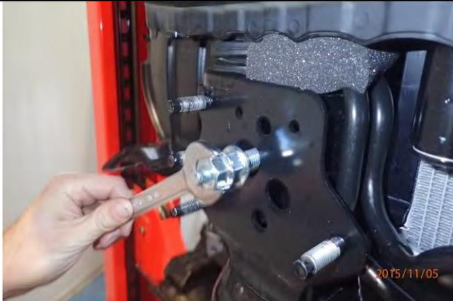
59. Install the chassis stud by fitting 2 nuts to the end of the stud and tightening until thread bottoms out.
