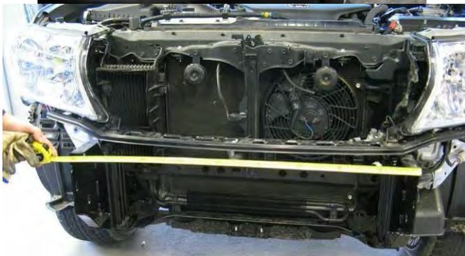
64. Tap the outer flange of the mount brackets until they are hard up against the tow hook mount area. Nip up the lowest outboard nut on each bracket. Brackets should be less than 935mm apart.
