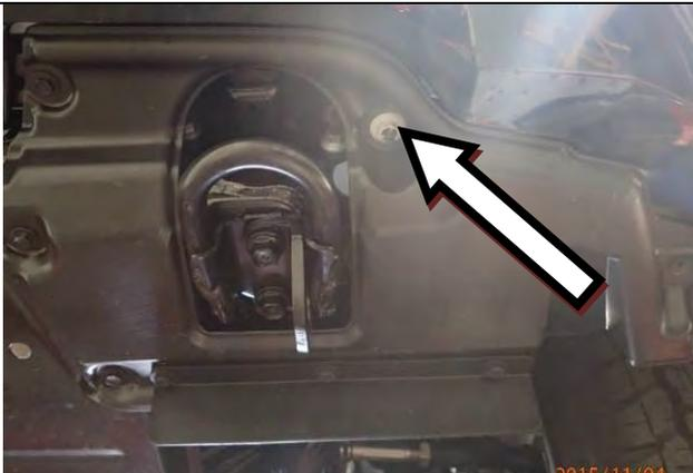
4. When removing lower trim panels, a plastic nut located on each side will need to be prised open with a small flat blade screwdriver to assist removal.
