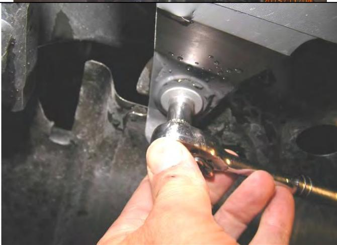
5. Remove lower bumper retaining screws.
