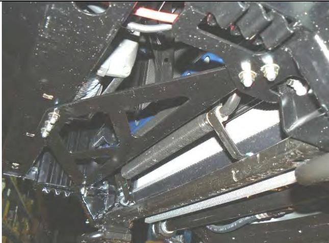
76. Loosely fit the cross brace to underside of lower pan and on top of gussets of mount brackets. Use M10 x 30mm SEMS bolt and flange nuts.
