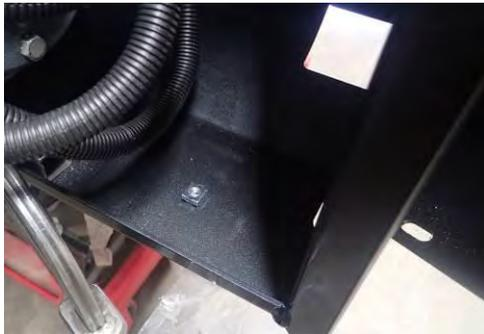
88. Fit the 4 longer leg M6 cage nuts to the lower pan of the bull bar as shown.
