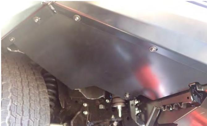
95. Trim the fender liner end flush with the splash panel face as shown. Then tuck the remaining wheel liner inside the wing panel return.
