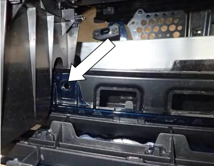
19. Remove plastic plugs securing upper bumper tabs to cross member.
