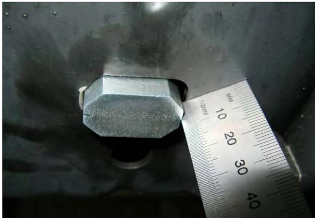
81. Then tighten up the long M12 chassis studs, ensuring that the clevis nut is positioned correctly over the hole in the chassis.
