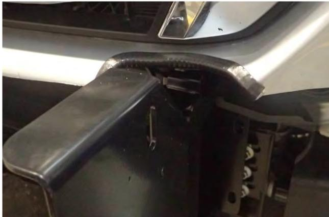
66. Fit pinch weld to the cut edge of the bumper as shown.
