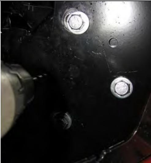
84. Using the M10 pilot holes in the bull bar uprights, drill the two pinning holes through mounting brackets on each side. Fit M10 bolt and washer sets and flange nuts and tighten to specified torque.
