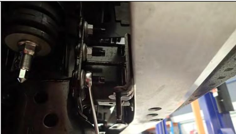
25. Remove foam absorber bar and set aside, this will not be reused
