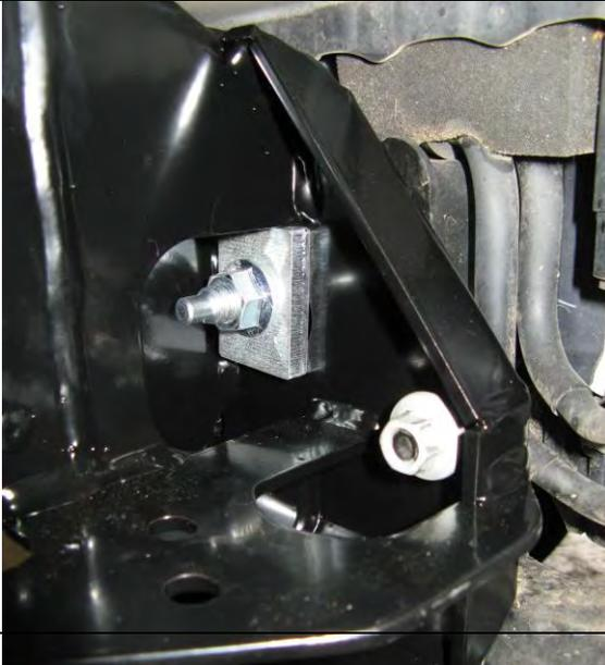
61. Loosely fit the mounting brackets to the chassis securing with the 8mm packers and flange nuts.
