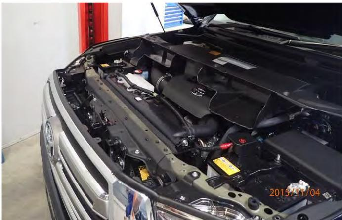
6. Remove plastic engine bay cover above grille area and set aside. Press down on centre of plastic plugs with small screwdriver or similar to release.
