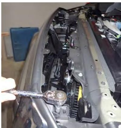
7. Remove retaining screws from top of grille
