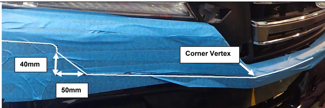
13. From where the template finishes, mark a line diagonally down, running 40mm down and 50mm across towards the centre of the vehicle as shown in picture.
