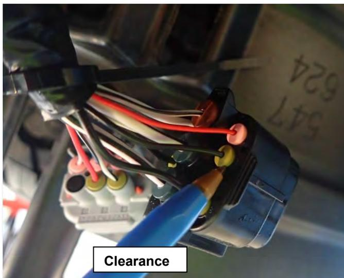
67. On the Driver's side Remove OE wiring loom bracket as shown with Phillips head screw driver. Detach plugs from bracket and discard bracket, it will not be reused.
