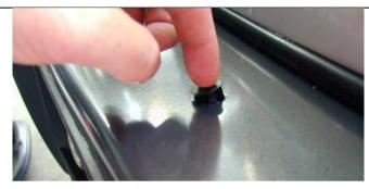
40. There are two Ø16 holes located on the top face of the bar. If no CB aerials are fitted the holes can be covered with the plastic plugs provided in the fitting kit.
