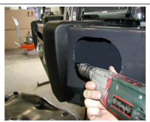
32. The bar must be pin bolted to the mount brackets. Using a drill and 10mm drill bit, drill through the upper and lower Ø10mm holes located in the mount brackets.
