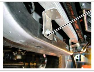
29. Bolt the deflector to the original bolts located in the chassis cross member.
