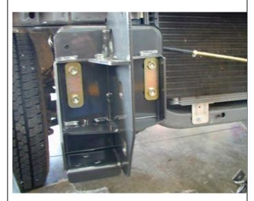
8. Fasten brackets with the M10 bolts, large 4mm thick washers, M10 spring washers, M10 flange nuts and plates, finger tight only.
