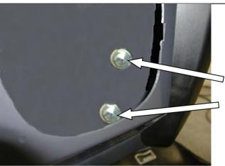
31. Bolt the bar to the mounts using M12 bolts, large flat washers and spring washers. Align the bar to the profile of the guards and tighten all bolts including the mount brackets.
