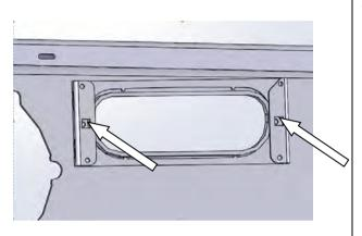
12. Install Nylon plugs (6821116). (4 off) Into Clearance Light/Turn Signal Brackets. (RH Shown).
