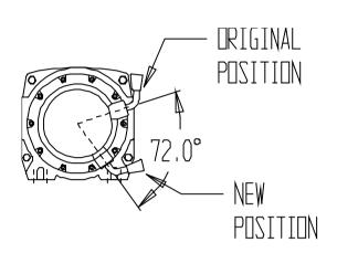
21. To place the winch clutch handle in a convenient location the winch gearbox must be rotated 2 hole spacing's, 72 degrees, in an clockwise direction when viewed from the gearbox end. Place the winch on its end and remove all gearbox bolts. Gently raise the gearbox just enough to rotate it. Do not completely remove the gearbox and avoid damaging the gasket. Refit all bolts and tighten.
