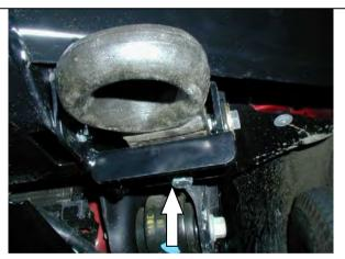
36. Bolt the tow hooks to the mount brackets using the M12 x 40mm bolts, flat washers and spring washers.
