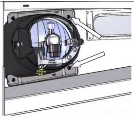
34. Secure into position as indicated using the 2 x fog lamp clamps and 4 x self-tapping screws.
