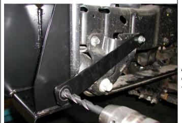
10. Bend the end of the strap inward, as shown, to allow the strap to sit against the bull bar mounting bracket.
