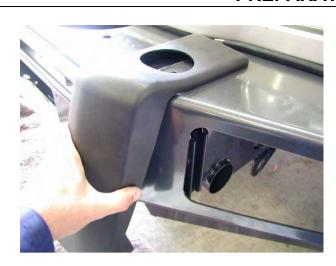
11. Insert the side buffers through the holes and fix using the M6 flange nuts. (LH Shown).
