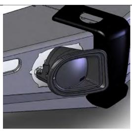
33. Fit fog lamp housings (3163082) into the bull-bar fog lamp cutouts as shown. (RH Shown).
