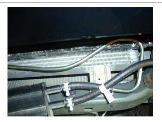
**IMPORTANT:**- When fitting a winch, on some models the top power steering cooler line (steel) will interfere with the winch and must be bent down to provide clearance as shown.
