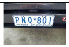
20. Bolt the number plate through the top holes using M6 X 16mm bolts and M6 flange nuts. If desired the double sided tape can be used down the sides of the number plate.
