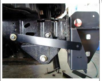
With the bull bar mounting brackets now in place (but not tightened) bolt the tension strap to the chassis using the hole next to the horizontal slot.
