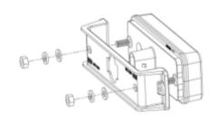
13. Install 6821285 bracket onto LED lamp with 2 x flat washer, 2 x spring washers and 2 x M6 nuts as shown.
