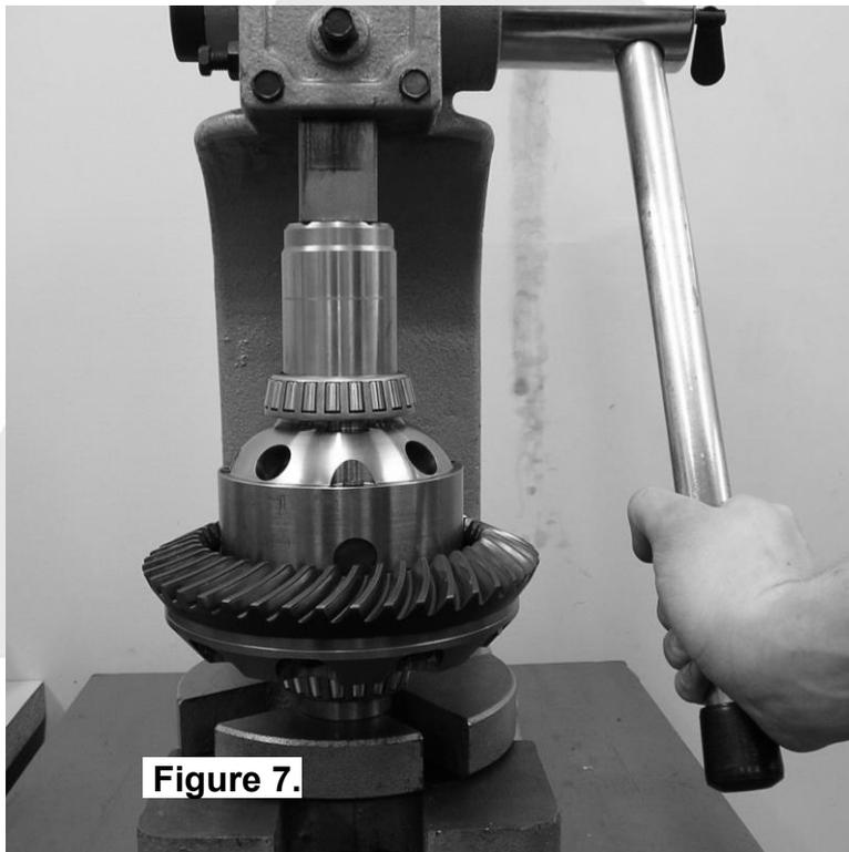
**NOTE :** Do not add any shims between the bearings and the bearing seat. Shimming of the *Air Locker* will be performed with the supplied shim kits and/or the OE master shims (if any) on the outside of the carrier bearings.
