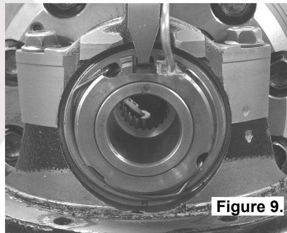
**NOTE :** Before attempting to install the adjuster nuts, make sure the threads on the inside of the bearing caps and differential housing are perfectly aligned. If they are not, the threads could be stripped.
