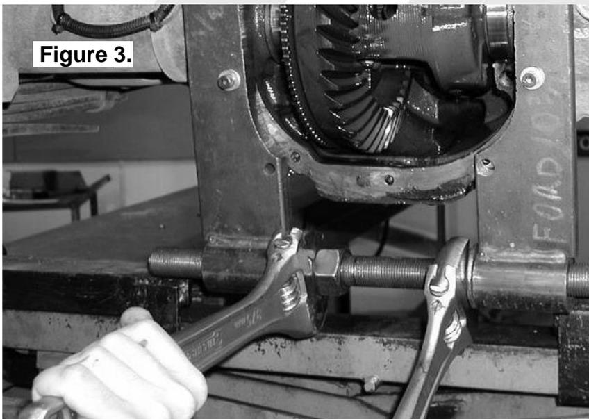
**NOTE :** The differential center is heavy and quite difficult to handle when covered in oil. Do not drop it!
