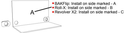
Assemble the clamping bracket loosely to the large end plates, for both passenger and driver sides.
