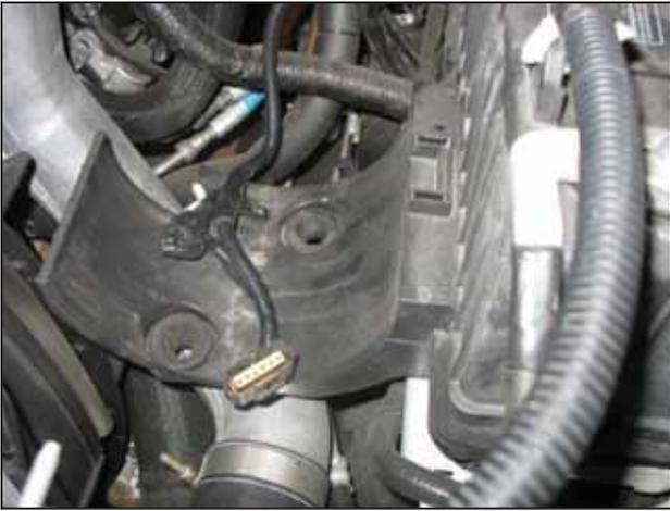
e. Pull up and remove the air filter housing from the engine bay.
