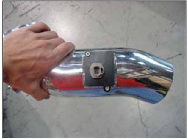
f. Install the IAT sensor into the grommet on the adapter plate as shown.
