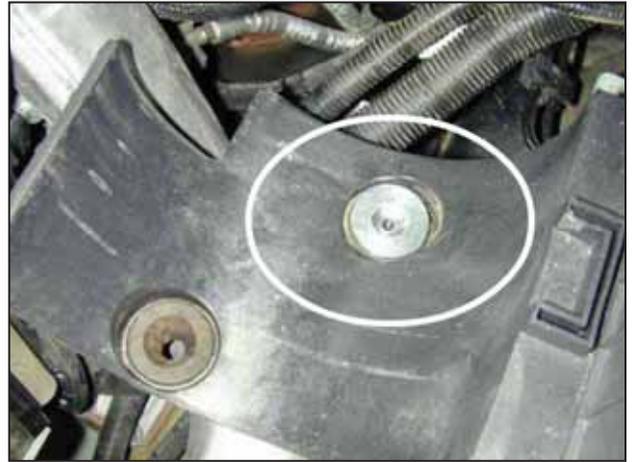
h. Install the billet aluminum stand into the rear rubber mount where the factory air box was removed.
