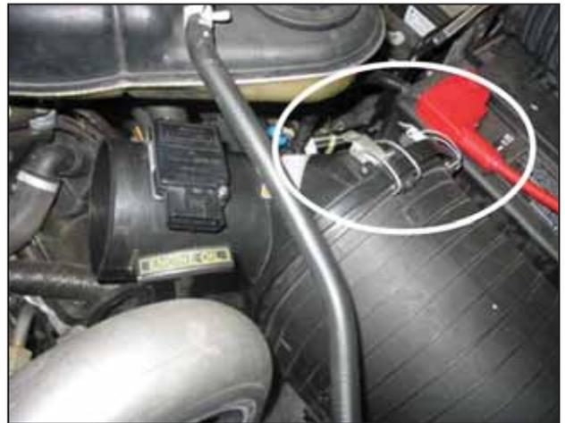
d. Unclasp the retaining clips holding the back side of the air filter housing together. Remove the rear side of the air filter housing by lifting up and pulling it out of the engine bay.
