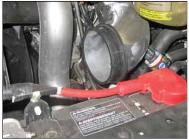
l. Install the supplied air filter adapter by stretching it over the filter end of the intake pipe.
