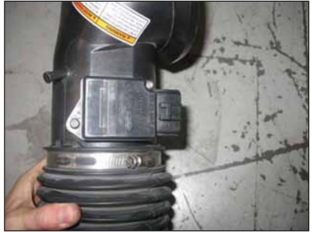
f. Remove the factory IAT sensor or MAF sensor from the stock air filter housing.
