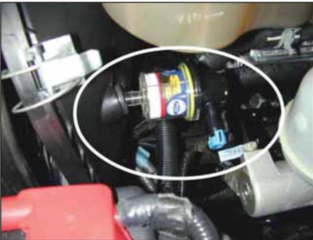
c. Unplug the wiring harness from the air filter restriction gauge. Remove the gauge from the rear of the air filter housing.
