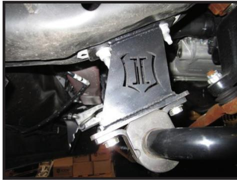
**24.** Using 3/8" hardware and a 9/16" socket/wrench, install the sway bar to the new drop brackets. [Torque to 33 ft-lbs]
