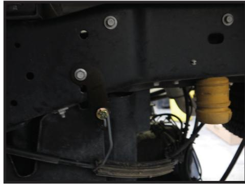
**28.** Using a 16mm wrench, unscrew the vent hose fitting from the axle tube. Fasten the bracket to the axle tube using the vent hose fitting (tighten 1/8 turn past snug). Fasten the brake lines to the bracket using the supplied 7/16" hardware. [FIGURE 10 & 11]
