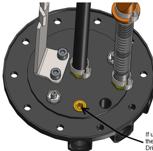
If using a returnless system where the ECU controls fuel pressure, Drill a 1/32" diameter hole thru the center of brass 1/8-NPT pipe plug.
