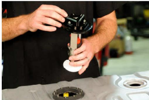
35. Press down firmly on the top of the pump assembly to compress the gasket. Start two of the 10-24 lock nuts on a pair of studs 180-degree apart. Tighten these two nuts until the remaining studs are approximately 1/4" exposed.
