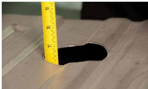
21. Measure the foam baffle assembly from the bottom (black rubber part) up and mark the assembly 1" longer than the determined tank depth. (If the tank was 6" deep, mark the foam baffle assembly to be 7" long)
