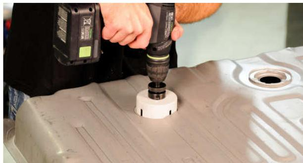
10. Place the included "installation ring" over the 3-1/4" hole so the raised register drops into it. Now rotate the ring until the bolt pattern is in the predetermined alignment. If the tank is corrugated or has ribs, rotate or clock the installation ring to ensure that none of the holes on the bolt pattern would have to be drilled into the side walls of the ribs.
