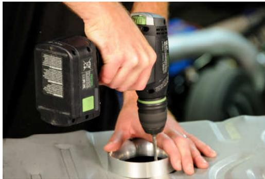
12. Place one of the included 10-24 x 2-1/2" screws in the above hole to help hold the index ring for further drilling.
