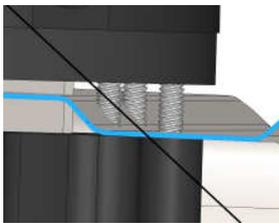
Avoid having mounting hole through side wall of rib.
