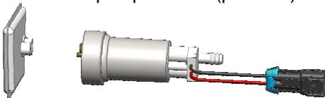
Position the fuel pump on the fuel pump hanger assembly such that from the bottom of the outlet cap to the bottom of the fuel pump strainer is equal to the fuel tank depth. Mark the bracket and the black outlet hose so they may be cut to the necessary lengths. Remember, take the time to measure twice and cut once!
