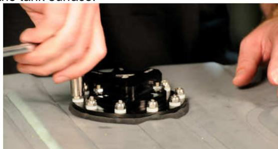
39. Prep the new tank by making all the necessary connection (feed, return, vent and electrical) before placing tank in vehicle. In most cases, once the tank is placed in the vehicle these connection will not be accessible. For electrical wiring refer to **Figure 2-1**.
