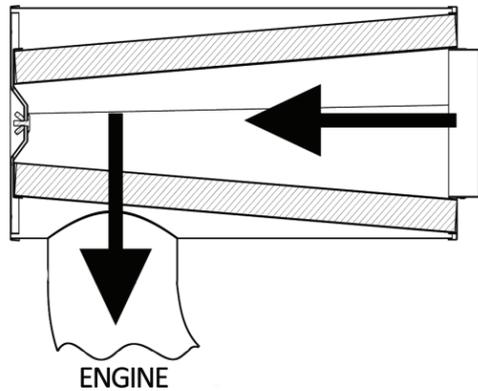
**CAUTION: THIS K&N® AIR FILTER ASSEMBLY SIZE IS AVAILABLE IN TWO DIFFERENT CONFIGURATIONS: STANDARD FLOW (S) AND REVERSE FLOW (R). BE SURE TO VERIFY THE AIR FLOW DIRECTION REQUIREMENTS OF YOUR VEHICLE BEFORE INSTALLING THIS K&N AIR FILTER ASSEMBLY. THIS K&N AIR FILTER ASSEMBLY IS A REVERSE FLOW ASSEMBLY AS SHOWN ABOVE (RED SIDE OF AIR FILTER, IS DIRTY SIDE).**
