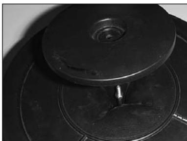
9) Place the Flow Control centering cap onto the Flow Control top.
