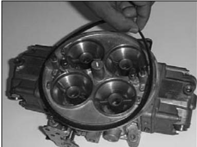
1) Apply the provided K&N gasket onto carburetor.
