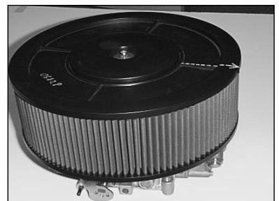
13) Once installation is completed, make sure that the arrow on the top plate is still facing in the proper direction.
