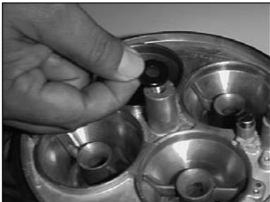
2) Apply spacer onto carburetor center post.
