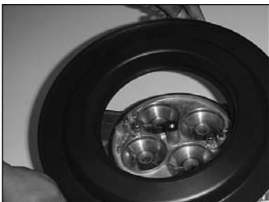
3) Place K&N base plate onto carburetor.
