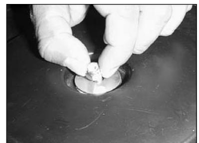
12) Place the provided nylock nut onto the stud and tighten down completely.
