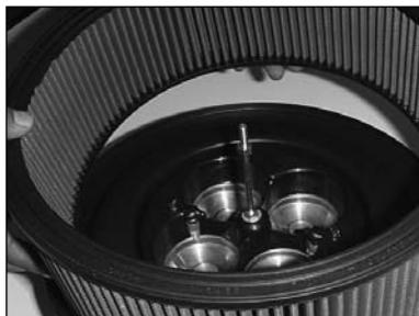
7) Place the K&N Filtercharger onto the base plate.
