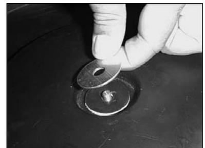
11) Place the provided large metal washer onto the stud.
