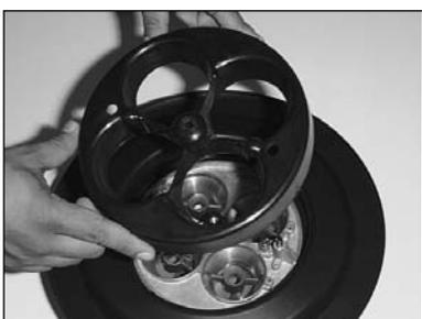
4) Place the K&N Flow Control Stub Stack onto base plate.
