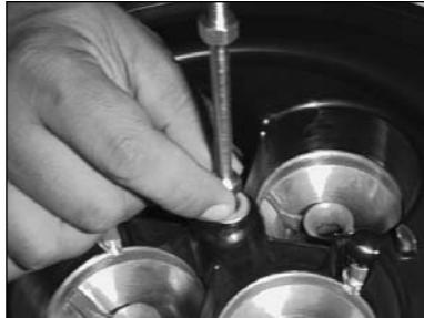
6) Place stud onto center post and tighten snug. **NOTE:** to avoid damage to the K&N Flow Control Stub Stack, do not over tighten.
