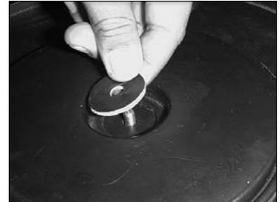
10) Place the provided black rubber washer onto the stud.
