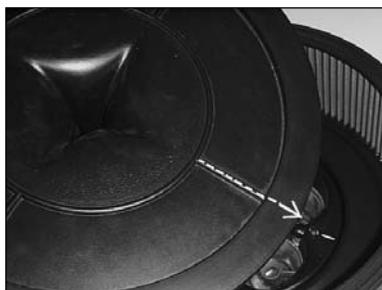
8) Place the Flow Control top onto the Filtercharger with the arrow pointing forwards or backwards to the float bowl vents.
