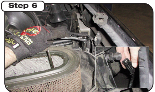
Using a 7/16" socket, remove nut securing lower air box half to engine compartment. Disconnect electrical harness going to temperature sensor on the side of the air box.
