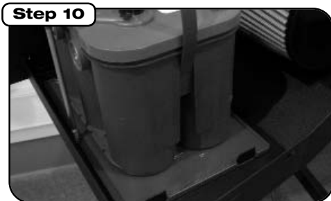
Install battery pad to housing. Place battery into intake housing using supplied clamp and two 8" long hex head bolts and locking washers. (DO NOT OVER TIGHTEN).
