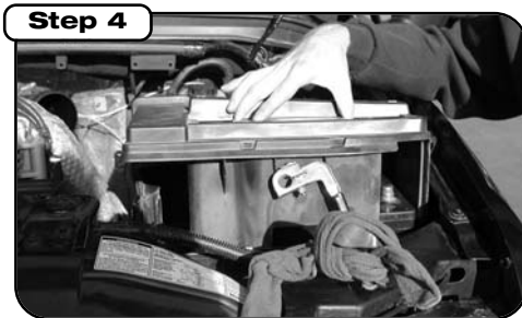
Remove battery terminals then remove battery lid. Wrap and isolate terminal or disconnect both batteries.
