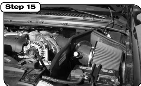
Place enclosed CARB EO sticker on a clean/smooth surface on or near the intake system. EO identification label is required in passing Smog Check inspection. Make sure all hoses and clamps are tight and that all electrical components are secure.
