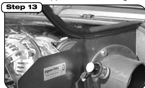
Install trim seal on housing.
