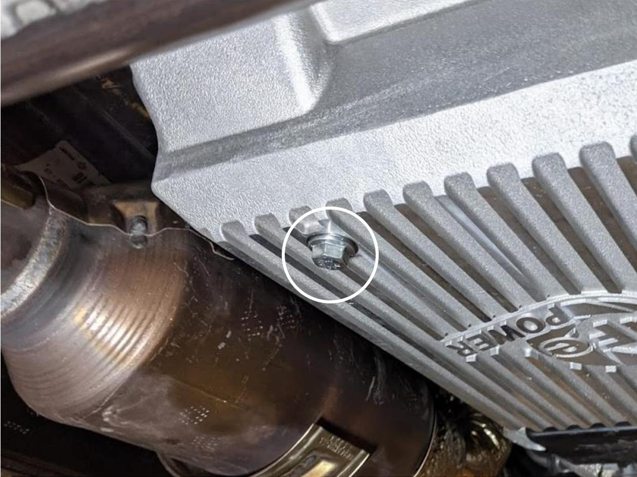
20. Hold the transmission pan up into position, aligning the bolt holes. Install one (1) M6x1.0x20 socket head screw and M6 washer into each of the four (4) corners to hold the pan into place.
