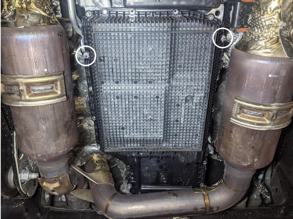
8. Once the fluid is pumped from the transmission, remove 18 screws from the pan, excluding the two (2) indicated near the front of the vehicle.
