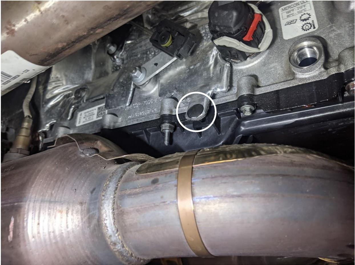
6. Using a pump, evacuate the remaining transmission fluid from the level port.
