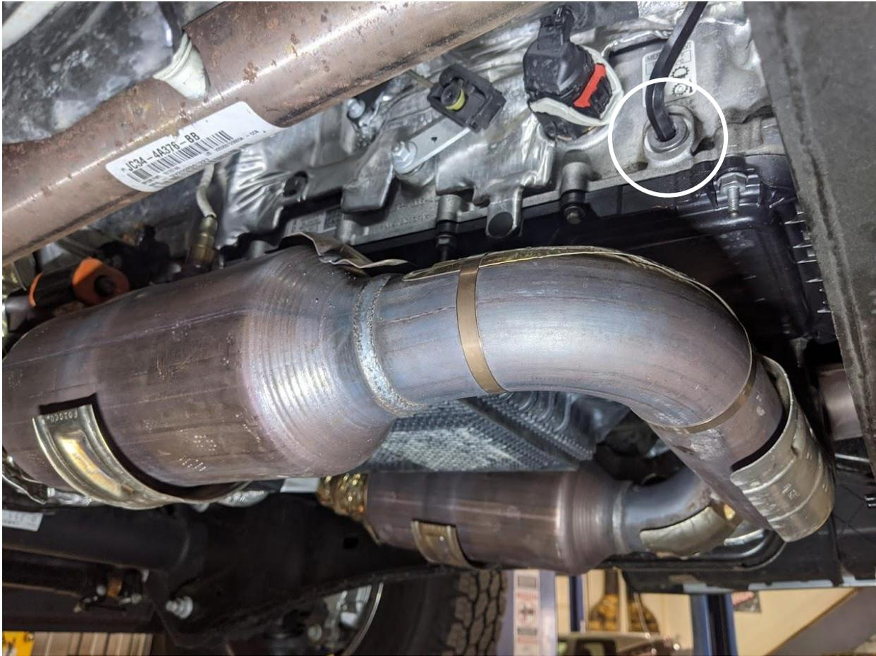
4. Position a large catch pan under the transmission pan.
