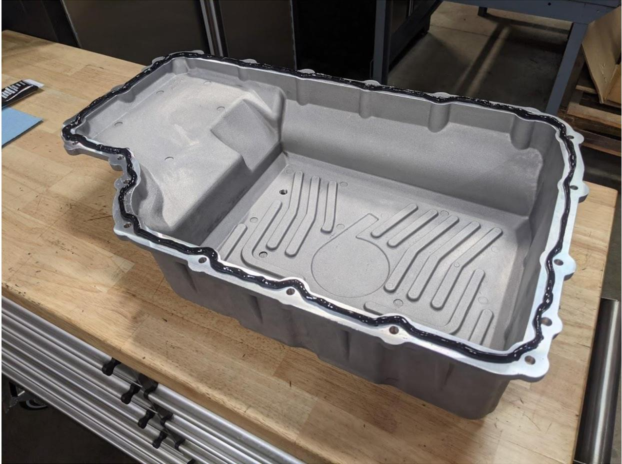
18. Once you have a clear path to lift the aFe transmission pan into place, prepare the 20 supplied M6x1.0x20 socket head screws and M6 washers.
