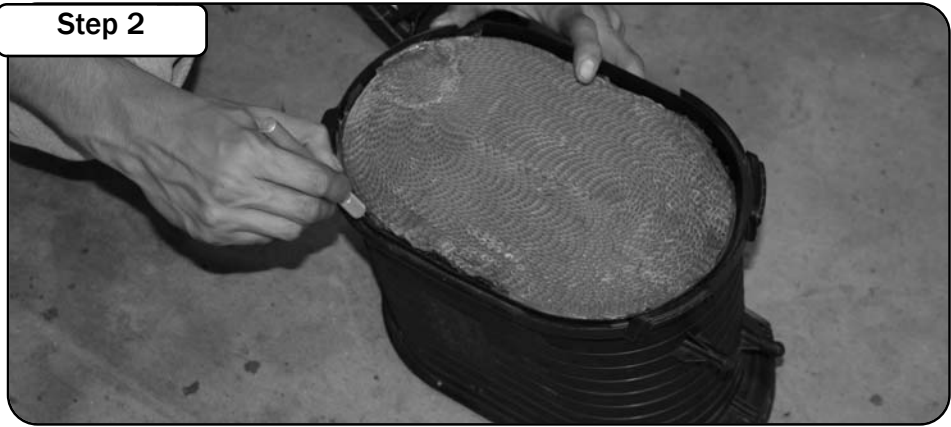
Step 2 With a knife or sharp blade carefully cut along the edge of the OE air filter from the side opposite seal. Discard the air filter internals.
