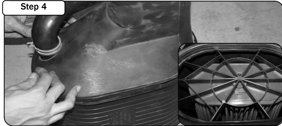
Step 4 Re-assemble the air filter assembly. Verify engagement grooves are positioned as shown to ensure correct installation. Reinstall assembly back into engine.
