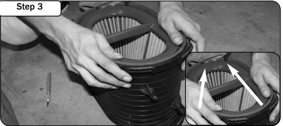
Step 3 Carefully slide the air filter into the canister as shown above. Pay close attention to the alignment of the mounting slots relative to the filter housing.
