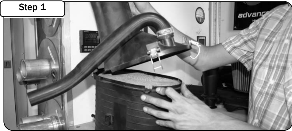
Step 1 Remove the intake system which includes the air filter. Separate the air filter from the intake system.
