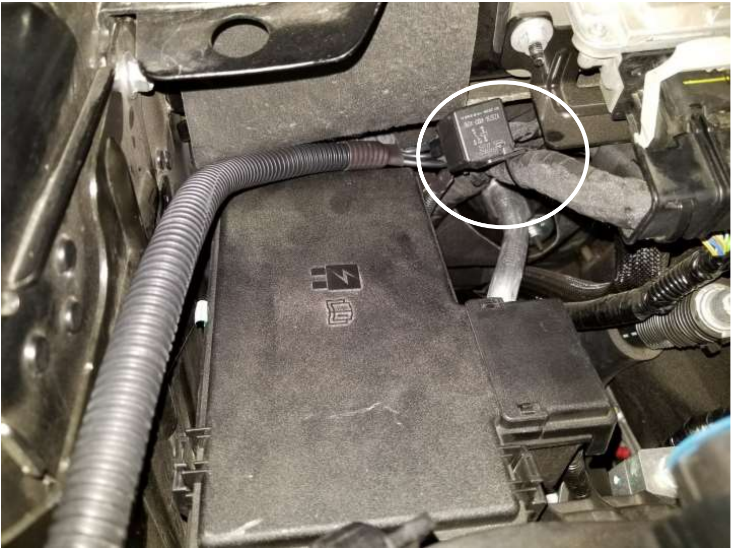
33. Secure the relay harness using a supplied nylon cable tie.
