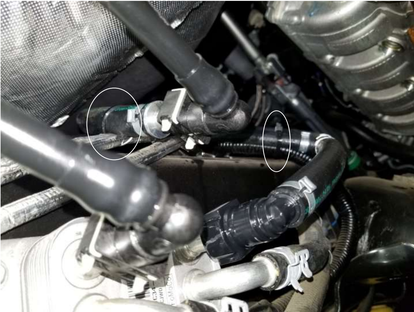
26. Using the supplied nylon cable ties, secure the new hoses (as shown above).
