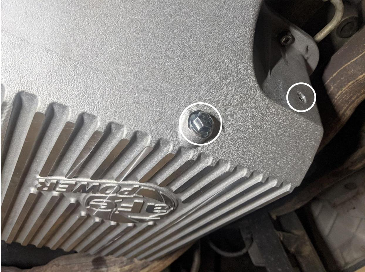
22. Install the supplied M12x1.25 magnetic drain plug and crush washer (secure about ½ turn past finger tight).
