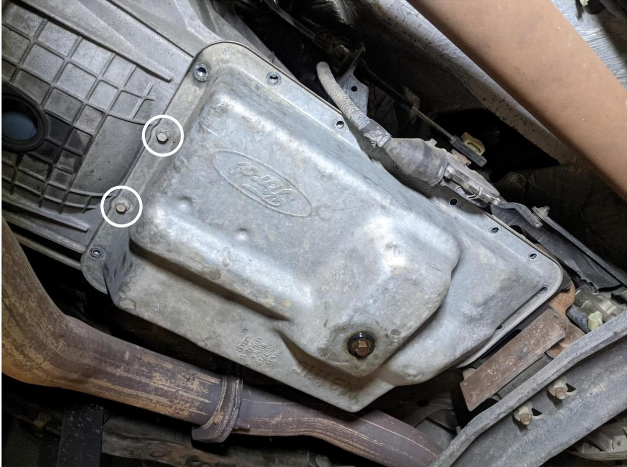
5. Remove 18 bolts from the transmission pan, leaving the front two (2) in place.
