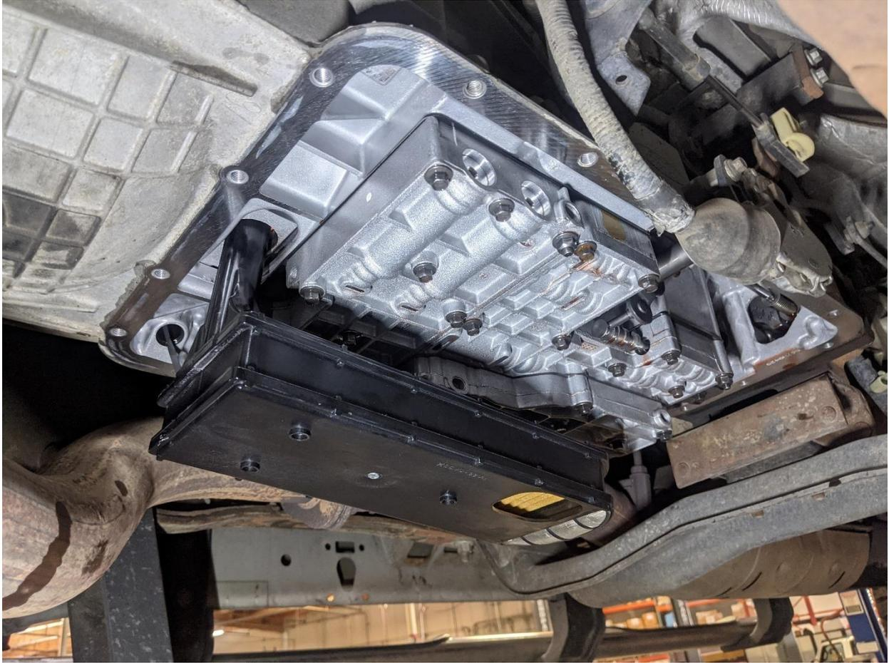
14. Install the supplied aFe transmission filter.
