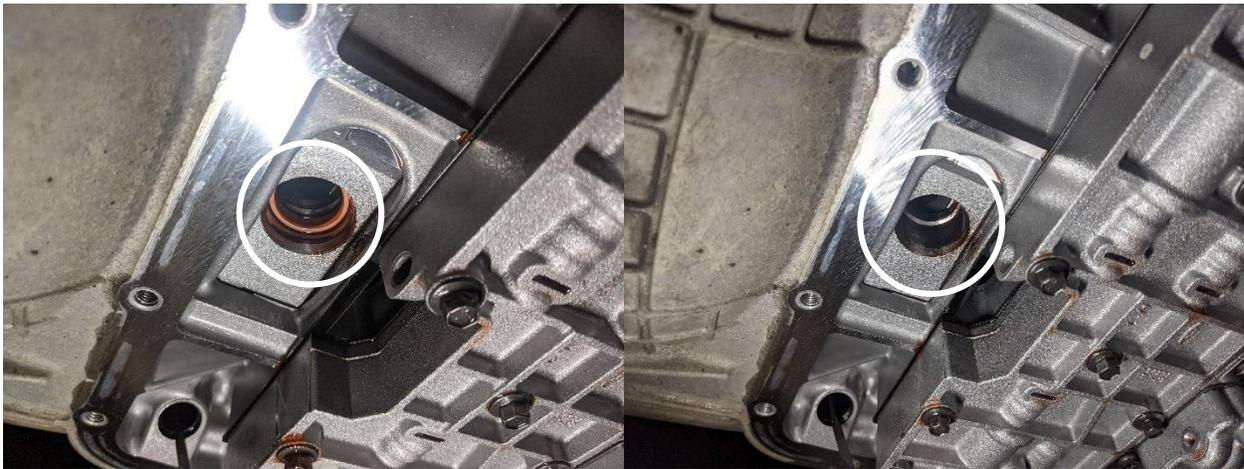
11. Clean the sealing surface with a gasket scraper. Be careful not to gouge the surface while cleaning.
