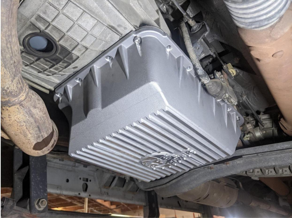
19. Hold the transmission pan up into position, aligning the screw holes. Install four (4) M8x1.25x20 socket head screws and M8 screws into each of the corners to hold the pan into position.
