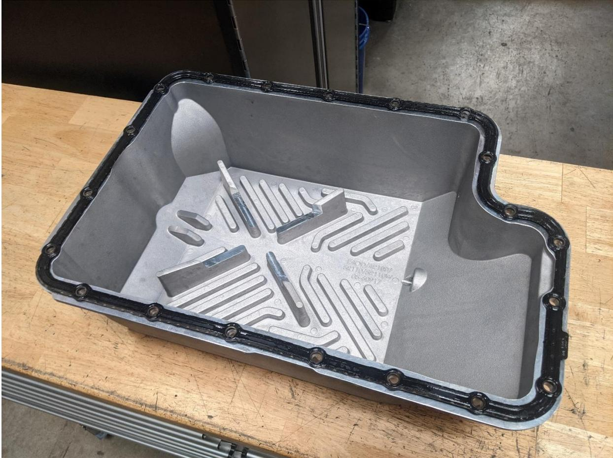
16. Hold the supplied aFe transmission pan up to the gasket surface to make sure you will be able to maneuver it into place.
