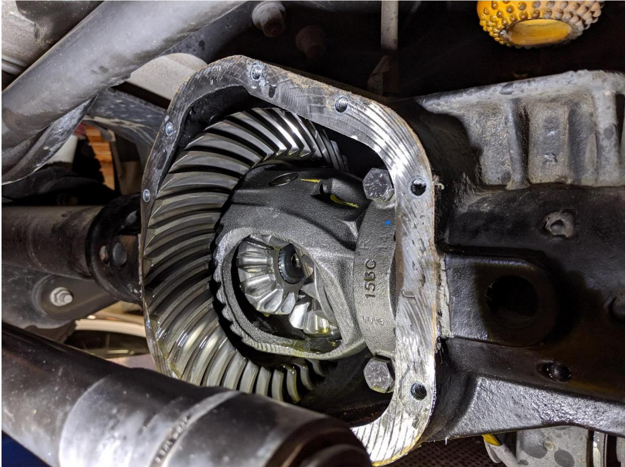
5. Allow all of the gear oil to drain from the differential.
