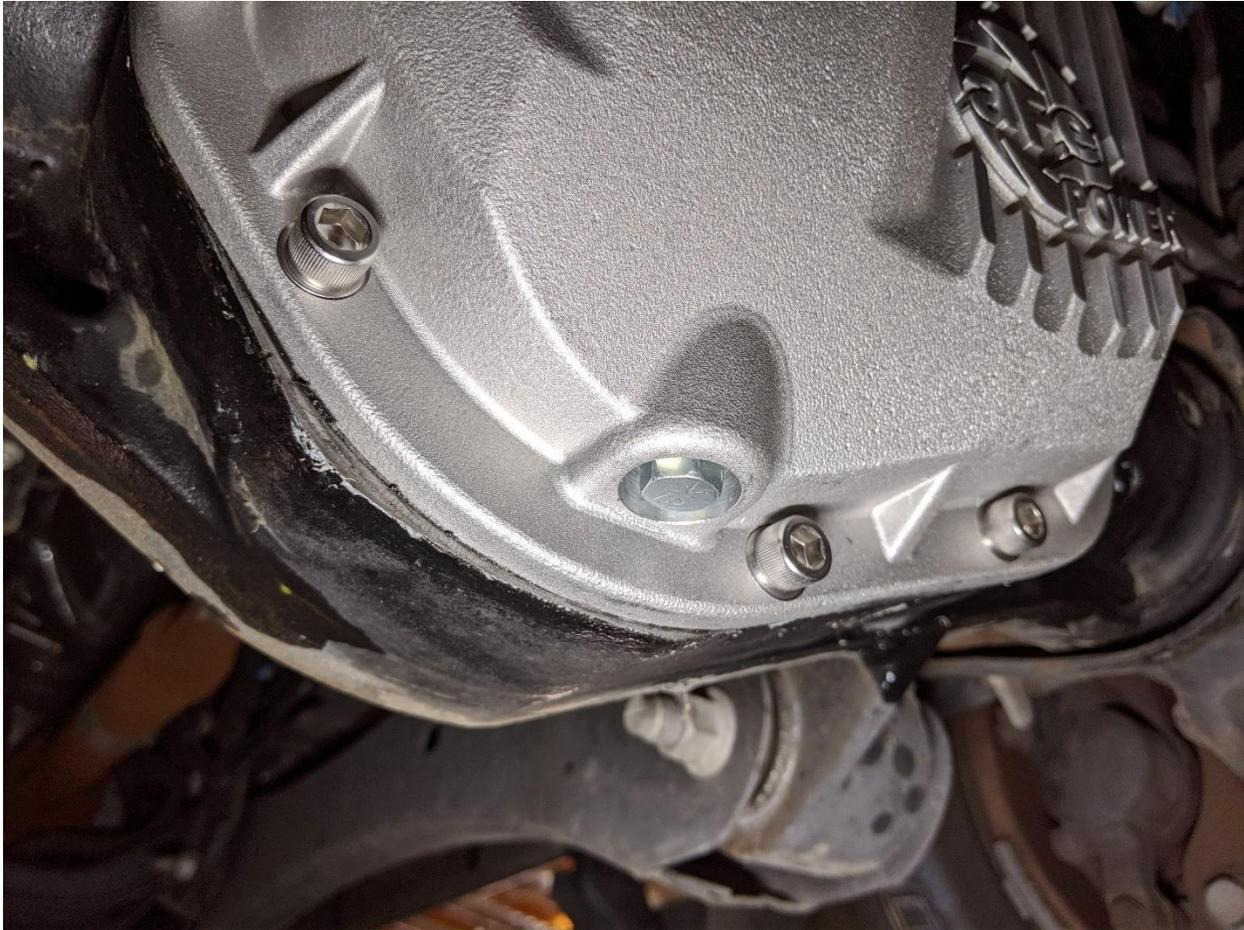
18. Install the supplied M12x1.25 drain plug and crush washer into the bottom of the cover.
