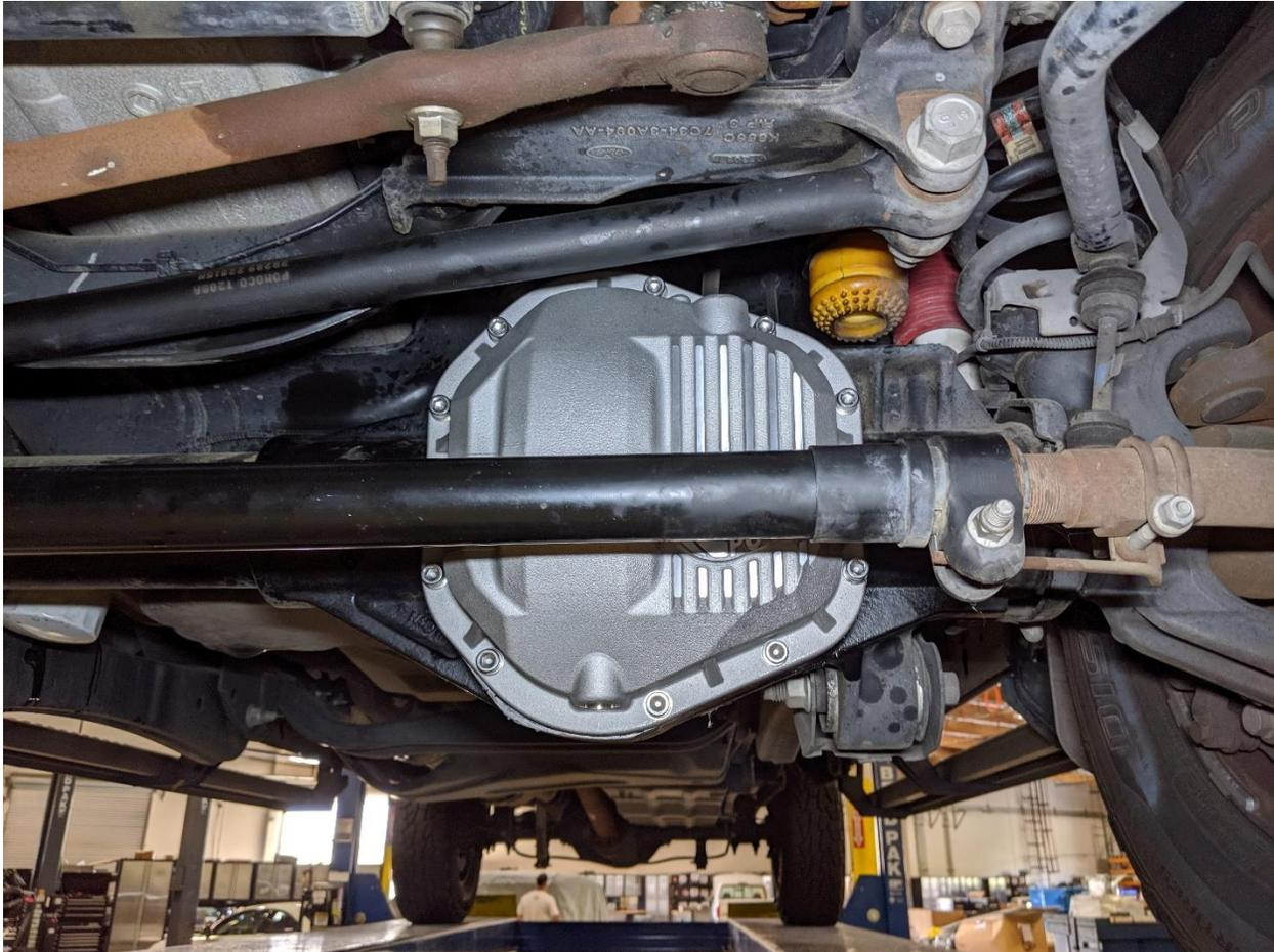
15. Hold the aFe differential cover into position, aligning the screw holes. Install four (4) of the supplied 3/8"-16x1" socket head screws and flat washers into separate sides of the cover to hold it in place.
