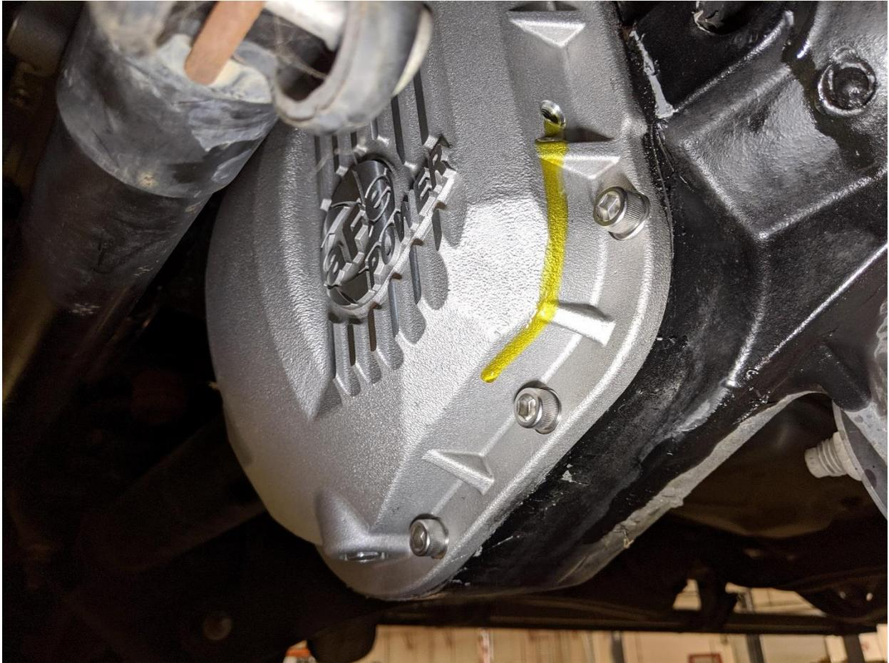
20. Using the top fill port, fill the aFe differential cover using new gear oil. Fill until gear oil runs out of the 1/8" NPT port on the side of the cover (about 4 quarts).
