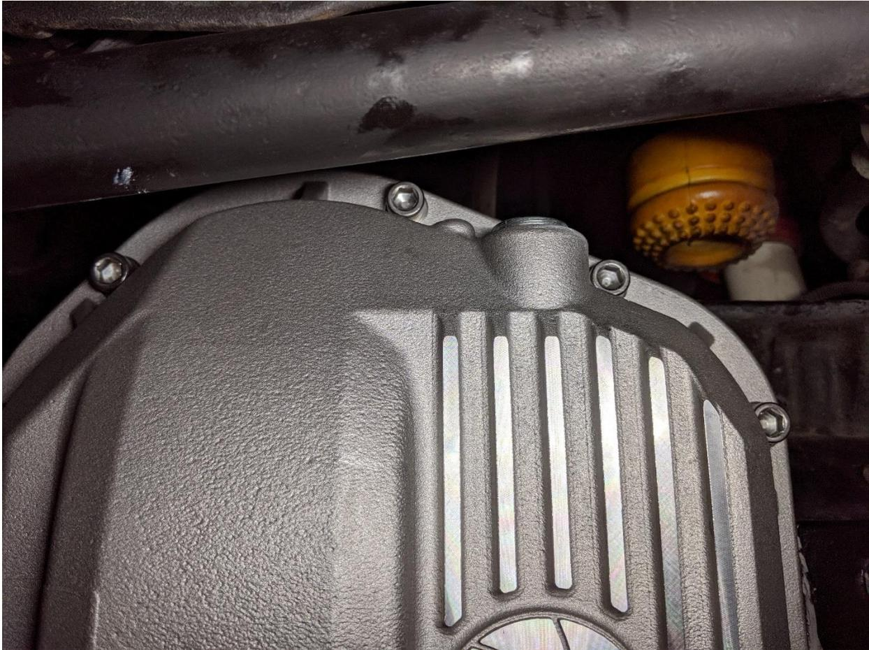
**Note: If your vehicle had a breather port attached directly to the differential cover, reinstall it now in place of the 1/8" NPT plug.**
