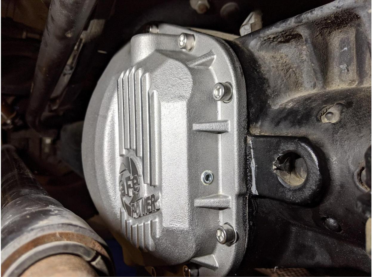
22. Install one (1) 1/8" NPT plug into the side of the cover.
