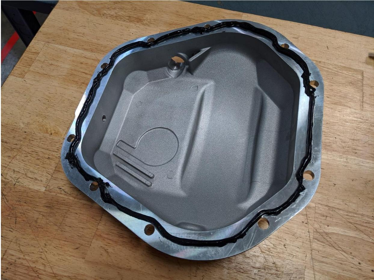
13. Hold the supplied aFe differential cover up to the gasket surface to make sure you will be able to maneuver it into place easily.
