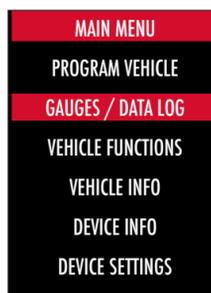
3. On **initial setup**, you will need to select **Configuration** press the center button, and select your vehicle from a list of data log files. In the future, you can continue without going through the vehicle selection.
