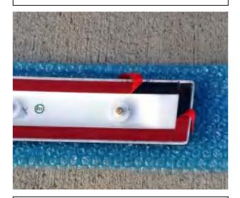
**STEP 3:** Peel back approximately 2" inches of protective tape liner, at alternating corners of the Body Side Molding, and fold to the outside at a 45 degree angle.
