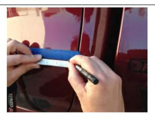
STEP 2: Position the Body Side Moldings onto the door to ensure an equal distance from rear back edge and front forward edge of the door, when aligned mark position with a non-permanent marker on masking tape. Ensure the correct Body Side Moldings are identified prior to installing to doors. Parts are identified on the back side of Body Side Moldings. (Left Hand Side shown above)
