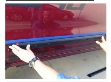
**STEP 4:** Aligning the rear end of Body Side Moldings with the position noted in step 2. Ensure the tape liners are facing outwards and apply light pressure in the exposed tape areas. If a ridge line is in door profile, position the Body Side Molding so the top edge of part runs below and parallel with the ridge line profile. (Left Hand Front shown above)
