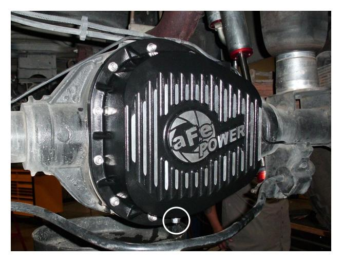
15. Install the supplied M12 x 1.25 drain plug and crush washer into the bottom of the cover (secure about  $\frac{1}{2}$  turn past finger tight).
