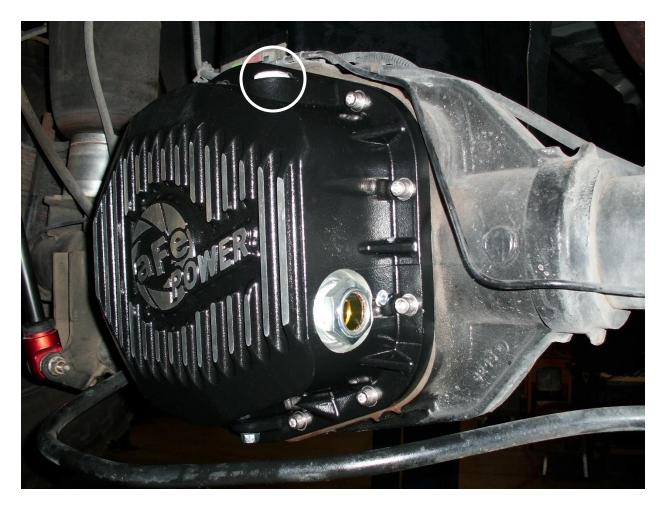
19. Apply Teflon tape/pipe sealant and install the supplied 3/4" NPT 6" Deep Reach plug into the top of the cover.
