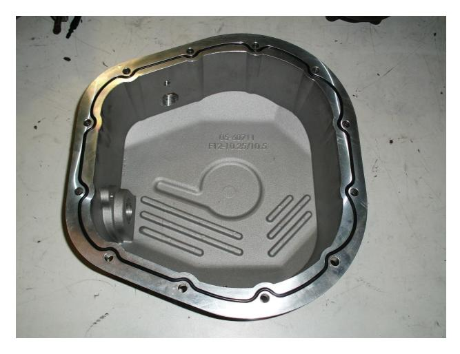
10. Lightly coat the supplied O-Ring with oil and install onto the provided aFe differential cover.
