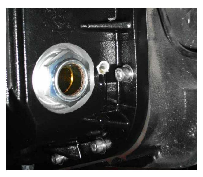
17. Using the top fill port, fill the aFe differential cover with new gear oil. Fill until gear oil runs out of the 1/8" NPT port on the side of the cover (about 5 quarts).
