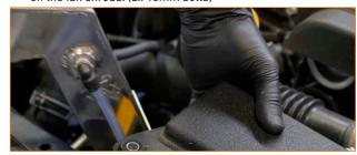
04. If you have a Mishimoto fan shroud installed on your vehicle, you will have to swap the original expansion tank bracket for the bracket included with your kit. Simply remove the two bolts that secure the original bracket and install the new one. (2x 10mm bolts)
