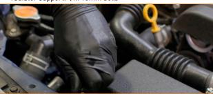
03. Remove the two bolts that secure the expansion tank to the fan shroud. Lift the corner of the intake resonator, and then remove the expansion tank by lifting it directly upward. The bottom of the expansion tank has a peg that fits into a bracket on the fan shroud. (2x 10mm bolts)
