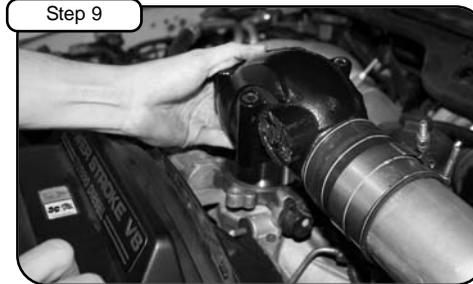
Carefully guide manifold into coupler hose.
