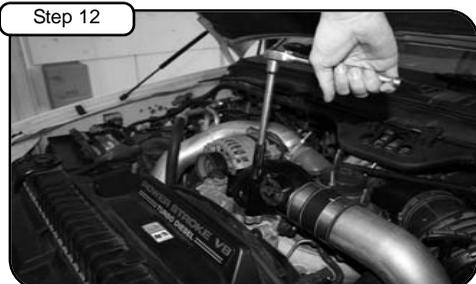
Tighten the four mounting screws from Step 11 using 10mm socket. See notes 2 & 5
