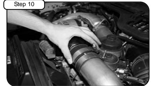
Slide back clamp. Do not tighten.
