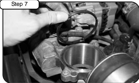
Remove old seal, replace with new seal provided.
