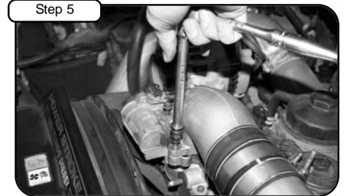
With 8mm socket and extension, loosen the 3 remaining screws.
