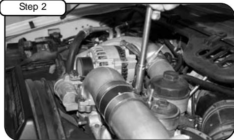
With a 7/16" socket with ratchet, loosen the intercooler coupler hose clamp. See note 6.
