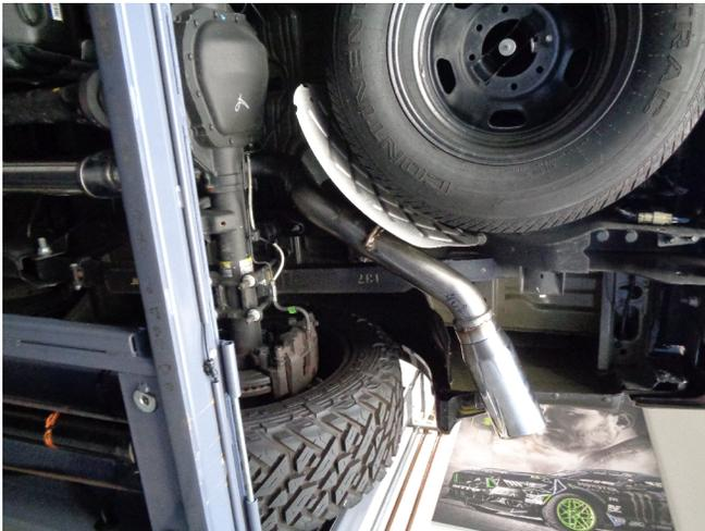
Step 6: Finish by loosely attaching the Tail Pipe Assembly using the supplied clamp. Install the welded hanger to the rubber insulator.
