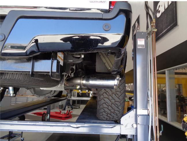
Step 7: Once a final position has been chosen for the new exhaust system, evenly tighten all clamps from front to rear using the torque specifications on page one of these instructions. Inspect all fasteners after 25-50 miles for operation and re-tighten if necessary.
