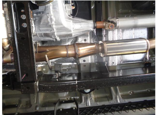
Step 4: Begin installing your new system by loosely attaching the Muffler Assembly to the catalytic converter outlet pipes using the OEM hardware. Engage the welded hanger to the rubber insulator.
