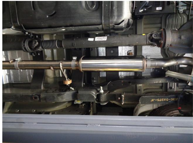
Step 5: At this point, if required, add the 19.25" Extension Pipe using a supplied clamp. Next, Loosely attach the Extension Pipe Assembly (has welded hangers attached) followed by the Muffler Assembly using the supplied clamps. Engage the welded hangers to the rubber insulators.
